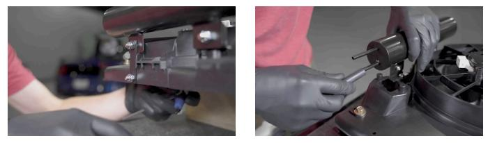
11. Insert lower fan bracket into s-clips, then align & secure upper fan bracket with supplied mounting bolts.
