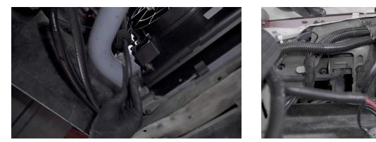
13. Install and wire supplied pig tails to power supply or fan controller of choice.
