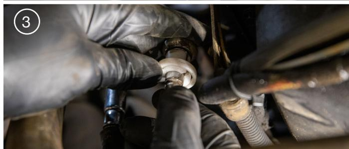
5. Remove factory plastic fuel hose from metal line. Use a sharp razor knife to cut through the factory plastic flex hose. This will allow you to peel back the hose and expose the factory barb connection on the metal fuel lines. (Figure 4)
