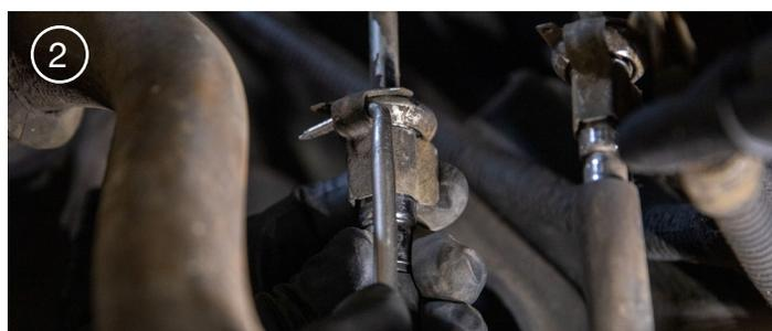
4. Use spring lock quick disconnect tools to release the retaining springs, then twist and pull at the joint to separate the connection. *(Be prepared to contain fuel with a shop towel and a catch pan.)* (Figure 3)
