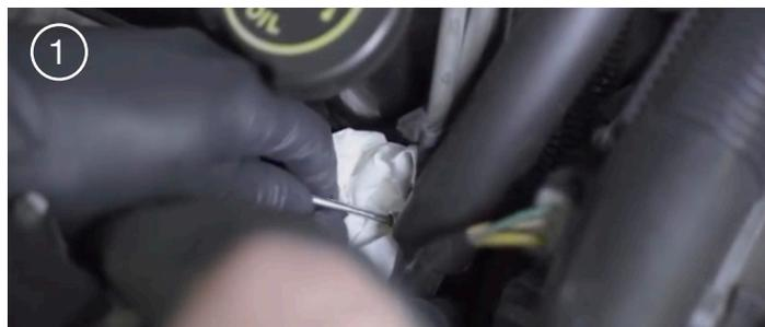
3. Use a small screwdriver or pry tool to remove the factory fuel line safety clips from connection joints. (Figure 2)
