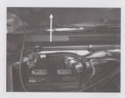
2. Lift up the plastic cowl cover to access the filter housing under it.
