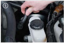
7. From within the fender well, reinstall and tighten the retaining nut for the factory proportioning valve.
