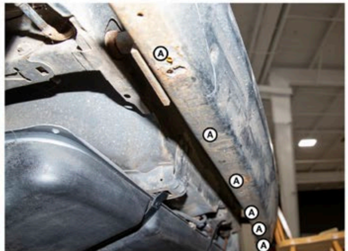
GT MODELS: PUSH PIN INSTALLS ON REINFORCEMENT BRACKET
