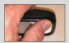
With the mirror in the frame, Push the frame into the housing until you feel it snap in place.
