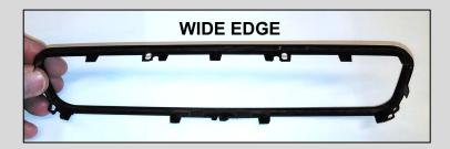
Install the mirror into the frame. The wide edge of the glass will go in the side of the frame shown in the picture. You can leave the lights out until the mirror is installed.
