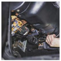
The large metal plate behind there has two 8mm screws, one on each side of the steering column. They are also holding the bottom of the instrument panel cover.
