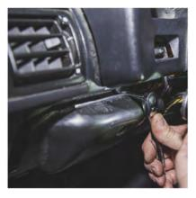
Remove the 7mm screws at the base of the windshield that hold the top of the instrument panel cover, then remove the instrument panel cover.
