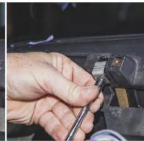
Use the supplied template to mark and drill a 3/16" hole for the larger LH bracket.
