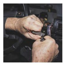
Take the supplied push-on J-nut and push onto the bottom side of the rectangular cut-out opposite of the damaged area being repaired. Mark and carefully drill a 3/16" hold in the center of the hole on the clip without damaging the surrounding plastic panel.
