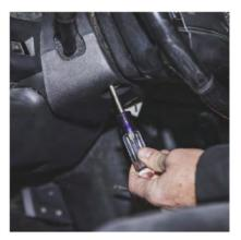
The lower plastic cover below the steering column has three 8mm screws and three push pin type fasteners along the bottom. Pull straight back towards the driver seat to release the clips.
