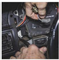
Pull out enough to release the two electrical plugs and the speedometer cable.
