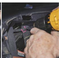
Insert the notched end of the bracket into the opening where the upper instrument panel cover screw goes & adjust until lined up with the drilled hole & top hole from instrument panel cover, then install the supplied screw into the drilled hole. Check alignment of instrument panel cover & reinstall removed parts.
