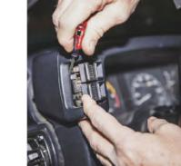
Next, the steering column cover has two screws on the bottom. Separate and set aside.
