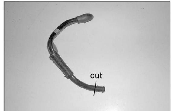
19. Cut the end off the idle air vent tube just below bead as shown. Then re-install vent tube back onto vehicle.
