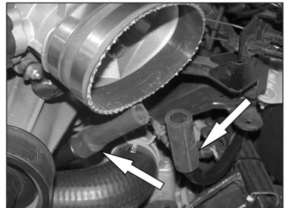
20. Install the two provide 5/8 silicone hoses onto the idle air and crank case vent lines as shown.
