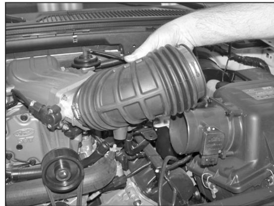
4. Remove the intake tube from vehicle.
