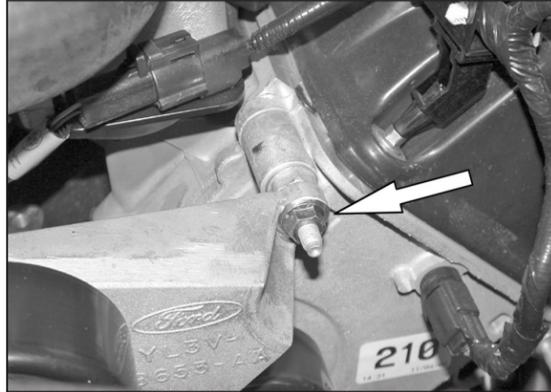
13. Remove the 8mm nut from stud that retains the idler pulley bracket.
