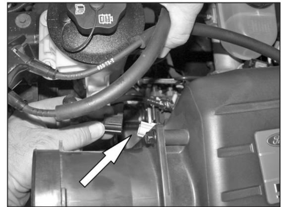
5. Disconnect the temp sensor electrical connection as shown.
