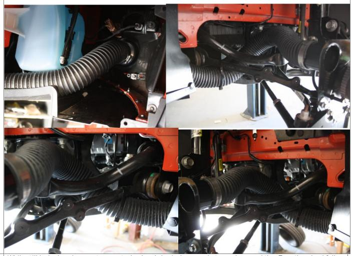
While still jacked up, be sure to mount wheel and check clearance between hose and tire. Turn the wheel full turns left and right.
