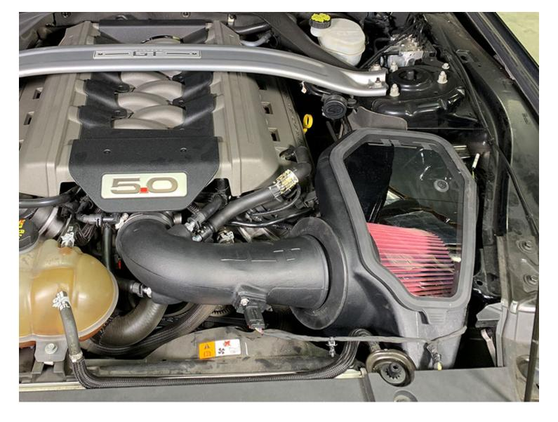
Inspect your installation, make sure the kit is properly positioned and all fasteners are secured. JLT recommends keeping all stock parts in case you would ever need to reinstall the stock intake. Affix the ID label near the intake kit. The installation is now complete.
