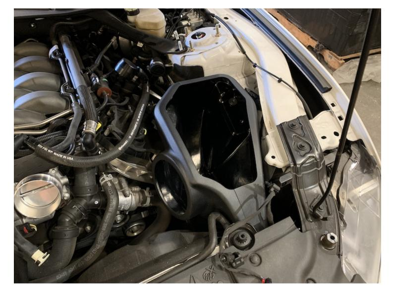
Place the JLT intake box (11) into the vehicle, ensuring that the front inlet completely encompasses the front grill air connection and that the prong found on the box seats snugly into the grommet shown in step 12.
