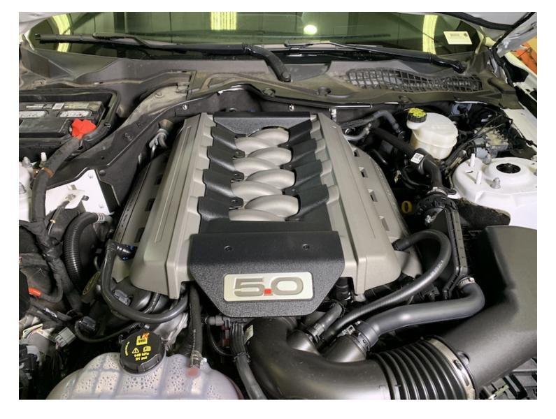
Lift up on the engine cover, popping it off of the top of the engine to gain access to the entire intake system.
