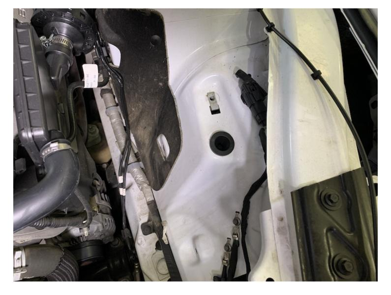
Verify that the grommet pictured did not come out of its hole on the vehicle with the stock intake box. If it did, remove it from the intake box and return it to its hole on the vehicle.
