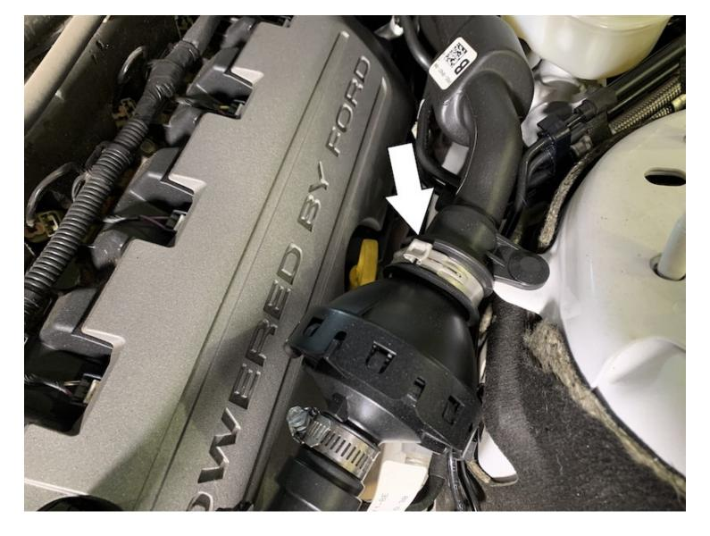
Cut off the crimp-on clamp shown on the cabin sound tube. After it has been cut off, remove from the vehicle, the section of the tube which used to connect the stock intake tube to the area where the clamp was found.
