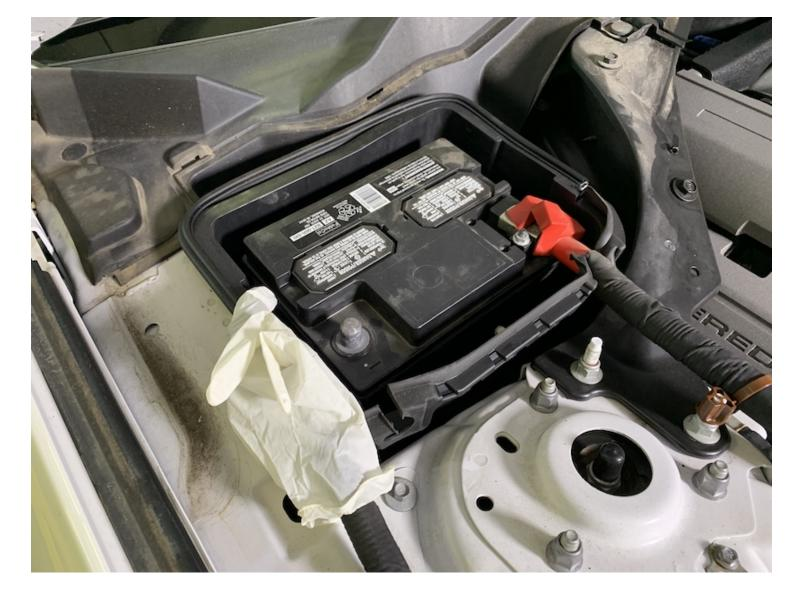
With the ignition switched off and the parking brake set, disconnect the negative battery harness on the battery. The battery must be disconnected for at least 2 hours to ensure proper functionality of the kit during use. Be sure to cover the end of the harness for the rest of the installation process.
