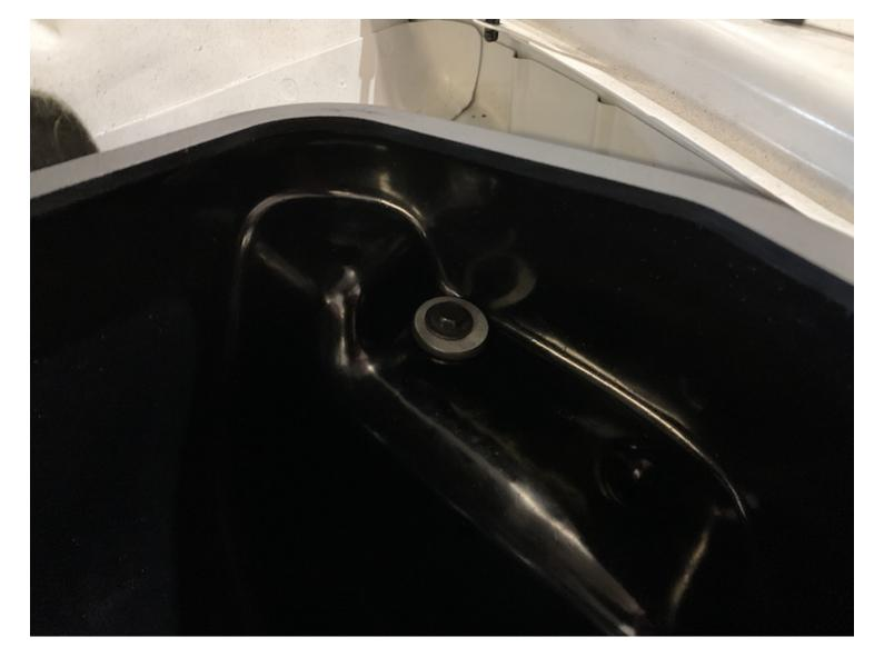
Secure the JLT intake box to the vehicle by reinstalling the screw removed in step 10.
