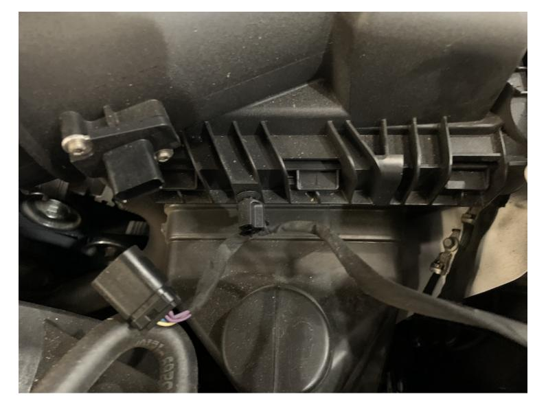
Pop off the MAF harness from it's mounting points on the stock intake box and vehicle frame.
