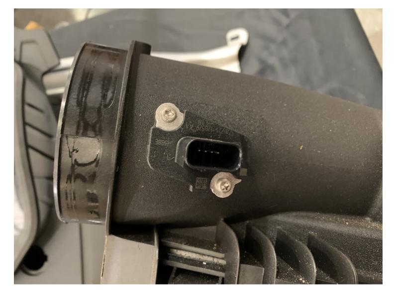
Remove the MAF sensor from the stock intake box.
