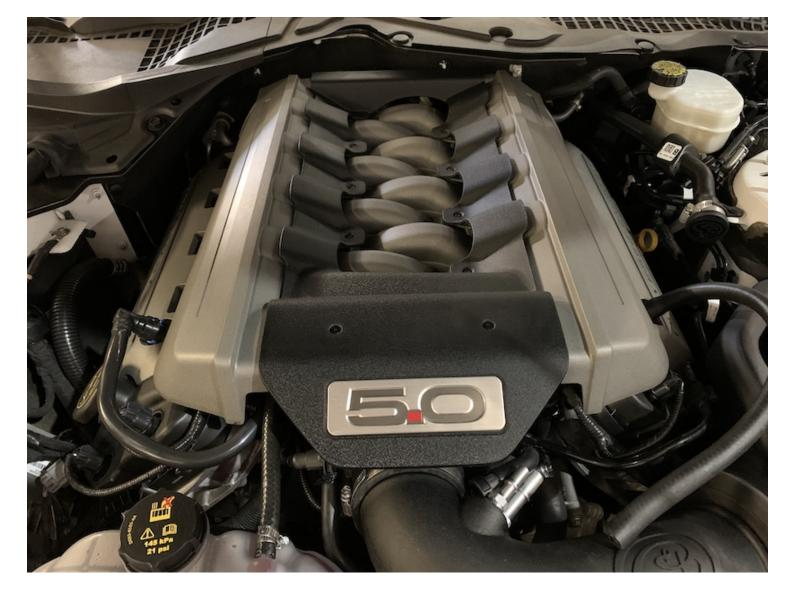
Reinstall the engine cover by pressing it down into the correct position on top of the engine.
