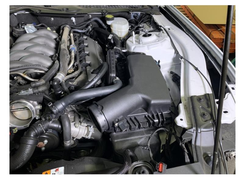
Remove the stock intake box from the vehicle by lifting it up and out.
