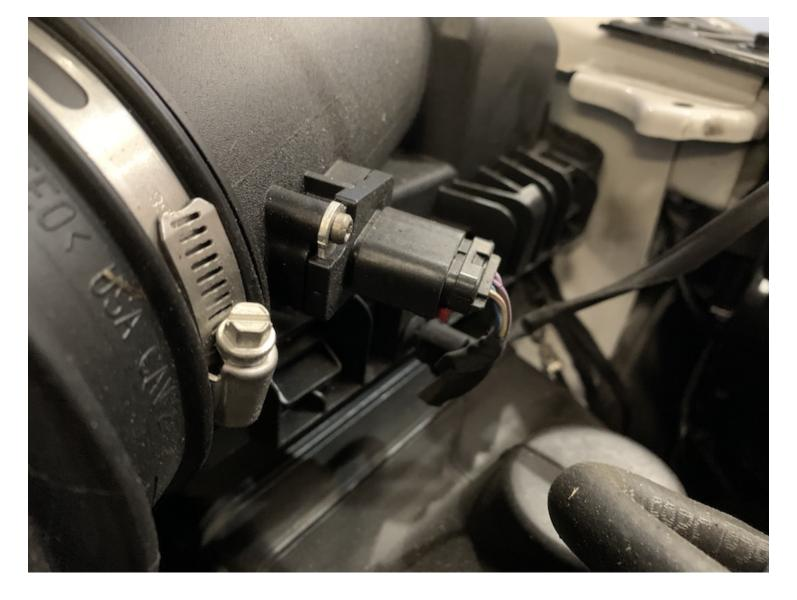
Pull out and push down on the red locking tab to disconnect the MAF sensor harness from the MAF sensor.
