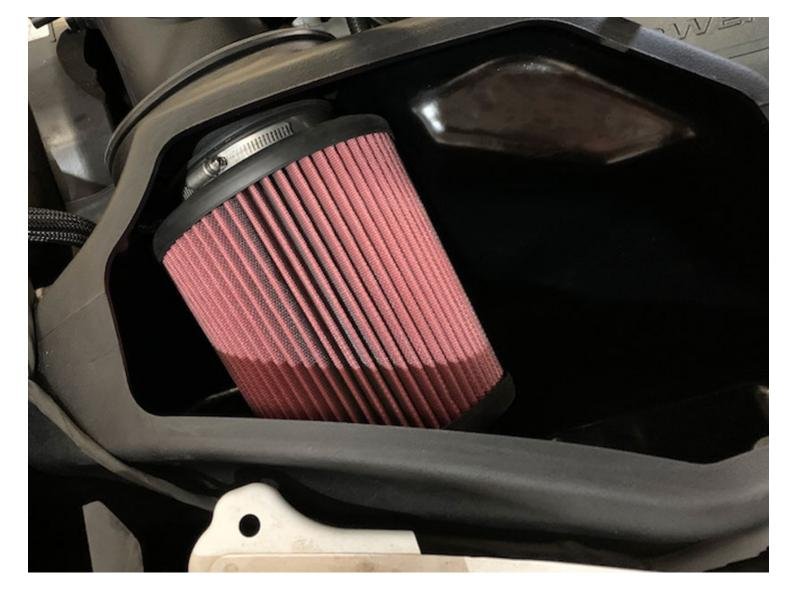
Connect the filter (10) to the JLT intake tube by placing it inside of the airbox and sliding the flange over the end of the tube. Secure the filter to the tube by tightening the #80 hose clamp (16).
