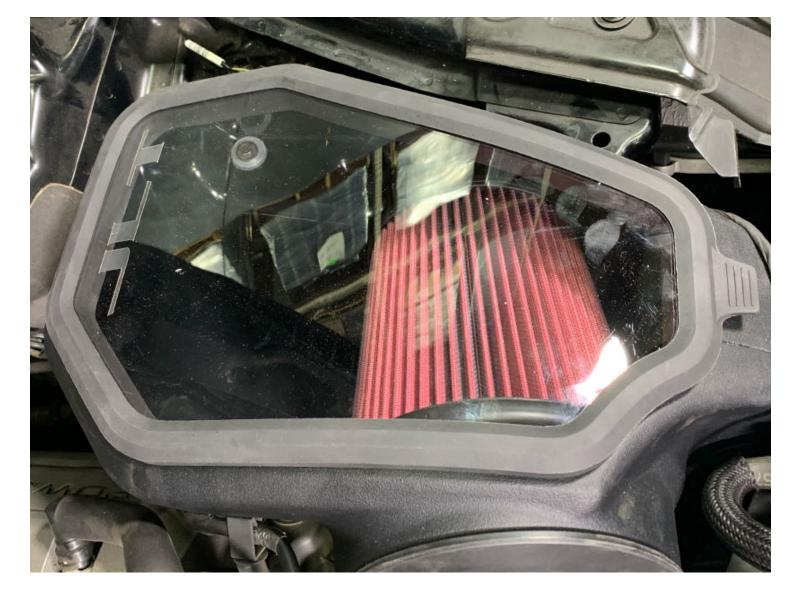
Install the lid seal (9) onto the lid (15) by stretching it around the perimeter of the lid. Snap the lid onto the top of the airbox by pressing down on all of the edges, ensuring that all edges of the lid are securely and completely snapped into place.
