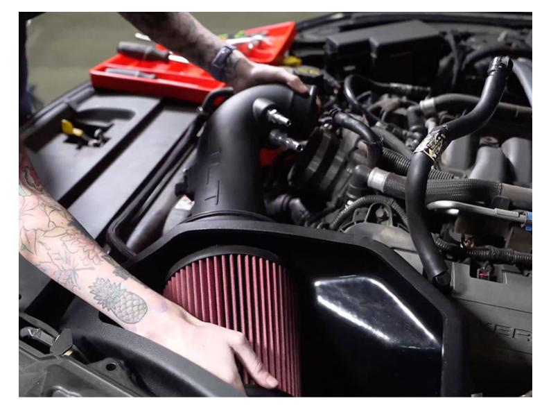
Install the S&B intake tube (12) into the vehicle in the position shown. Tighten the #60 hose clamp, securing the JLT intake tube to the engine throttle body.
