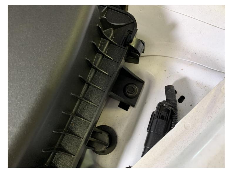
Remove the screw securing the stock intake box to the vehicle.
