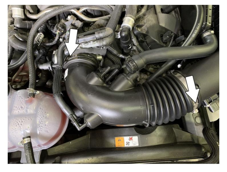
Loosen the hose clamps found on both ends of the stock intake tube. Remove the tube from the vehicle.
