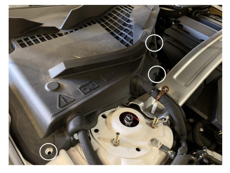
Remove the battery cover from the vehicle by removing the twist on panel screws in the 3 locations shown. To remove each screw, rotate the heads counter clockwise for a few rotations and then lift up.
