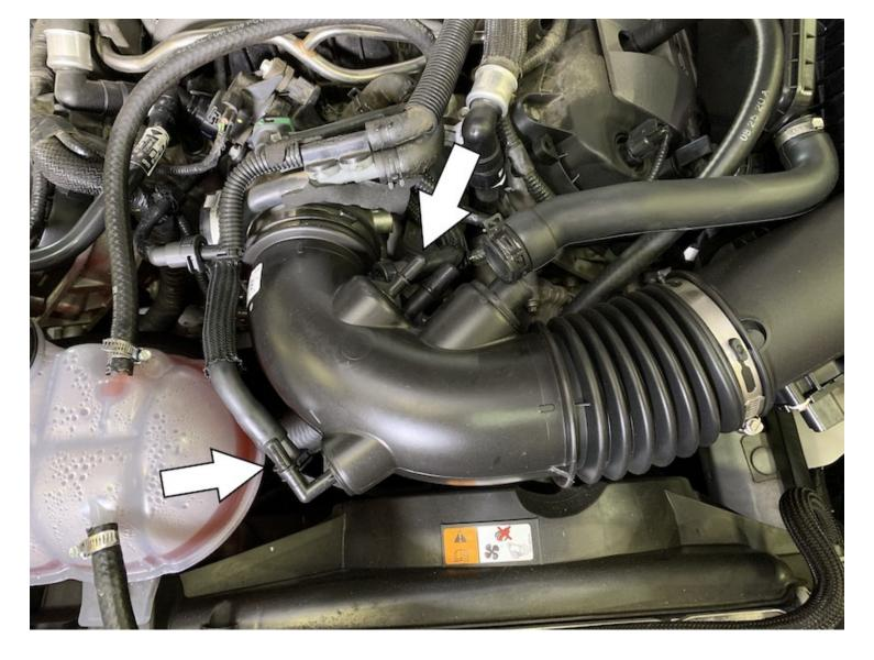
Disconnect the two indicated hoses from the stock intake tube by pushing the black tabs in and pulling out. If you have the 2017 model year, your intake tube will not have the connection found closer to the engine.
