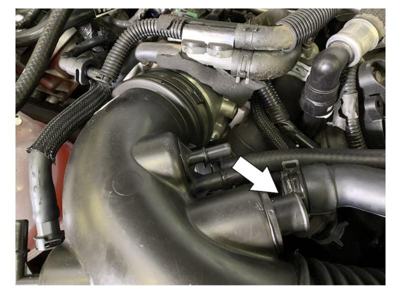
Disconnect the cabin sound tube from the stock intake tube by squeezing the clamp with pliers and pulling out.
