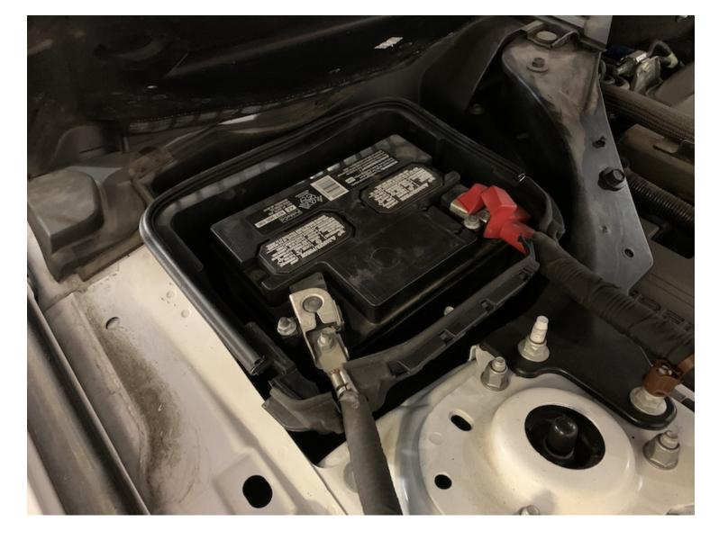
Reconnect the negative terminal on the battery.
