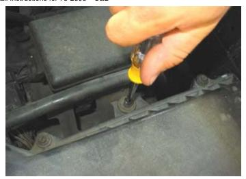
Remove vent hose from airbox and valve cover.
