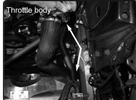
2. Loosen the clamp on the throttle body using 7mm nut driver. Loosen the clamp on the intercooler side also.
