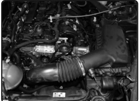
1. Remove the factory intake system or injen intake system from vehicle for installation of the new intercooler pipes. (See *injen instruction sheet PF9091*.)
