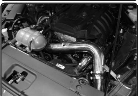
**23.** Re-install the intake system or stock air box. Make sure to connect the crankcase line and diverter valve return line. PF9091P intake system shown above.
