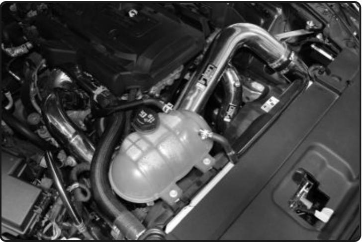
Congratulations! You have just completed the installation of this intercooler pipe system. Periodically, check the alignment of the intake, normal wear and tear can cause nuts and bolts to come loose. **Note: Check clearance and adjust if needed! Failure to check the alignment and adjust the intake can cause damage that will void the warranty. Injen Technology is not responsible for any damages caused by/from improper installation.**
