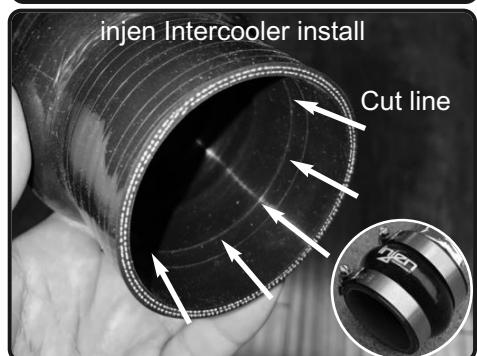
**17.** With injen Intercooler only, locate inside the hump hose for the cut indicator line. Cut back the intercooler hose at this 1" line. This will allow for the hump hose to be 2.5" x 2.5"L. **Cut only with injen intercooler only!**
