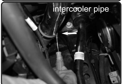
**20.** With soap water lubrication on the inside of the hump hose. This will allow for the elbow hose to slide on easier to intercooler. Tighten clamp using 8mm nut driver.
