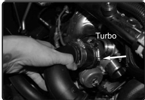
10. Pull back the intercooler pipe from turbo.
