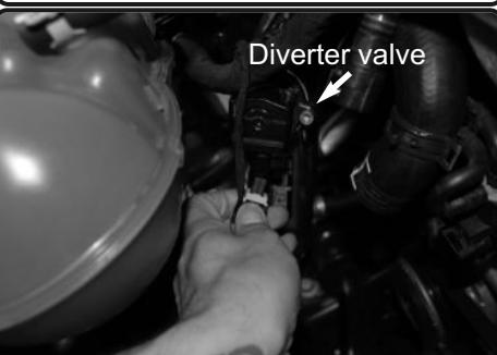
**22.** Re-connect the diverter valve harness.
