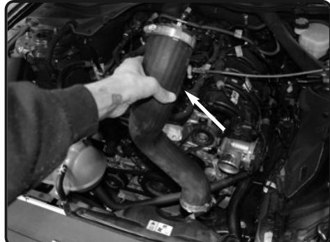
7. Carefully pull out the OEM rubber cold side intercooler hose out of vehicle.
