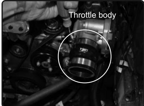
3. Install the provided 2-3/4" hump hose to the throttle body using provided clamps, tighten the clamp on throttle body only.
