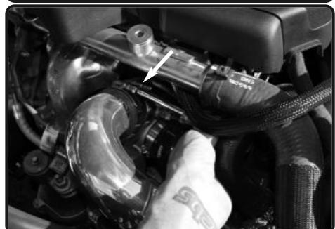
**21.** Secure the turbo side of the coupler and tighten using 8mm nut driver.
