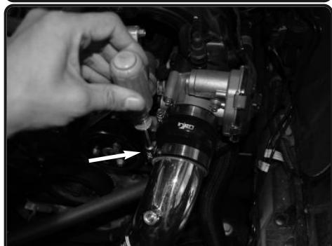
4. Secure the threaded fitting on intercooler tube if not using for auxiliary boost/injection line with provided 1/8" NPT plug. Secure and tighten. Install the provided 2-1/2" elbow hose to the intake tube with clamps provided.
