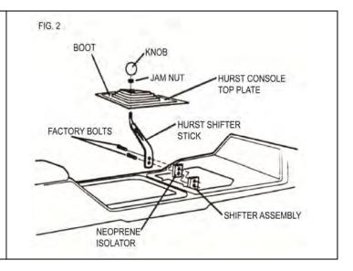
3. Place the console top plate over the shifter and slide the boot down over the stick. Position the top plate onto the console and carefully push down until the top plate is flush with the console and firmly in place.
