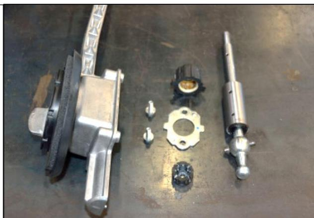
32. Apply the provided grease to the large factory pivot cup and snap it into place on the large ball portion of the Indy Shifter.
