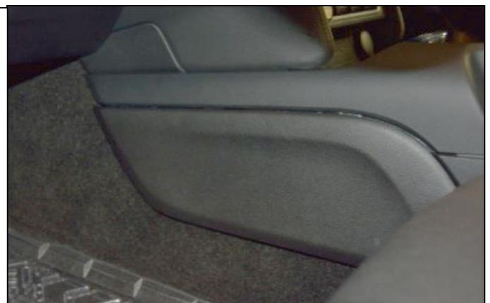
49. Install the factory shift boot onto the reverse lockout. There are three threaded holes in the upper portion of the lockout align the notches on the shift boot to the holes on the reverse lockout and push the shift boot down into place.
