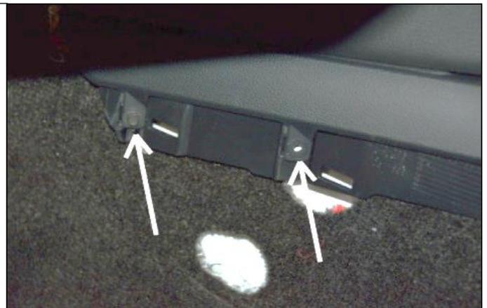
48. Re-install the front driver side and passenger side panels from the center console.
