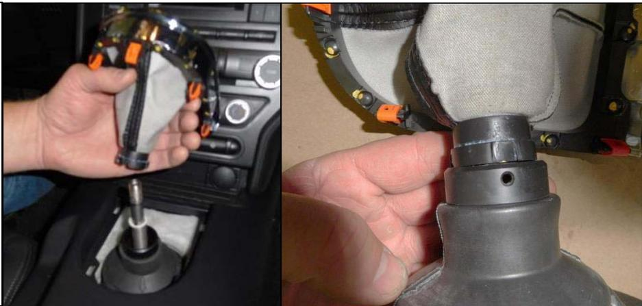
50. Install the three supplied set screws and evenly tighten the shift boot into place.
