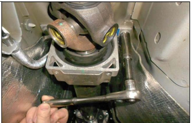
18. Once the center bearing bolts have been removed, you can pull the driveshaft back and lower the front end of the driveshaft. Allow the driveshaft to rest on top of the exhaust.
