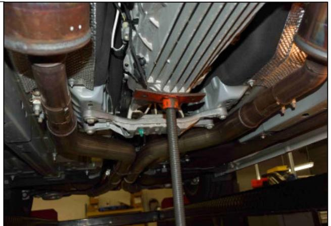
14. Remove the four (4) 18mm bolts securing the transmission to the frame. Lower the rear of the transmission. Support the rear with a transmission stand if you have the vehicle supported with a lift; support the rear with a floor jack if you have the vehicle supported with jack stands.
