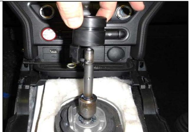
41. Align the reverse lockout block to the threaded hole on the larger portion of the Indy shifter. Use the retaining screw that was removed in step 9 to secure the reverse lockout into position.
