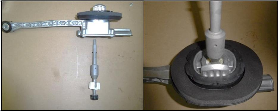
35. Seat the large pivot cup aligning the two tabs to the two recessed slots in the bottom of the shifter housing.
