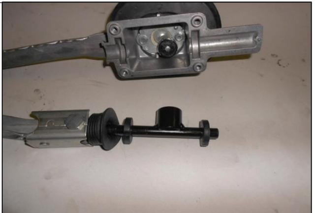
30. Remove the shifter retaining plate from the bottom of the shifter housing.
