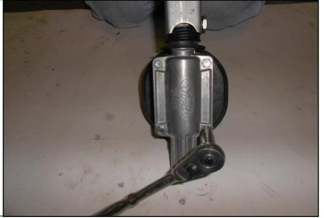
27. Remove the bottom Plate. Take care when removing the bottom plate, there is a rubber gasket that will be reused.
