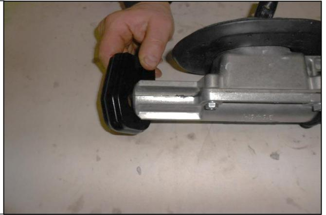
38. Insert it into the bracket clip. You will need to form the clip bracket around the new bushing to make it easier for install. The holes need to be 4.21 inches apart to be re-installed. It will be improbable that you will get it to hold at 4.21 inches apart, but try to get it close to 4.21 inches as possible. You will rely on a pair of channel locks to compress the assembly during install.
