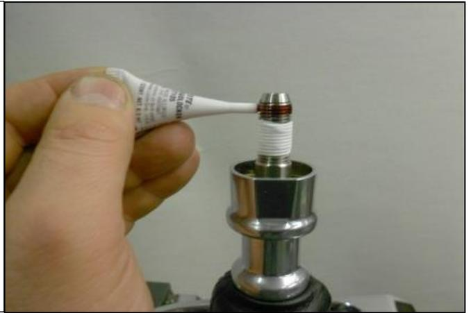
54. Screw knob onto handle until the bottom of the knob is just even with the top of the lockout collar (see photo). Continue to screw the knob an additional one turn plus whatever is necessary to align the shift pattern/logo properly.
