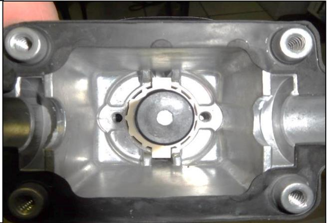
36. Reinstall the shifter retaining plate. The plate should seat flat against the bottom of the shifter housing. Torque to the factory specifications.
