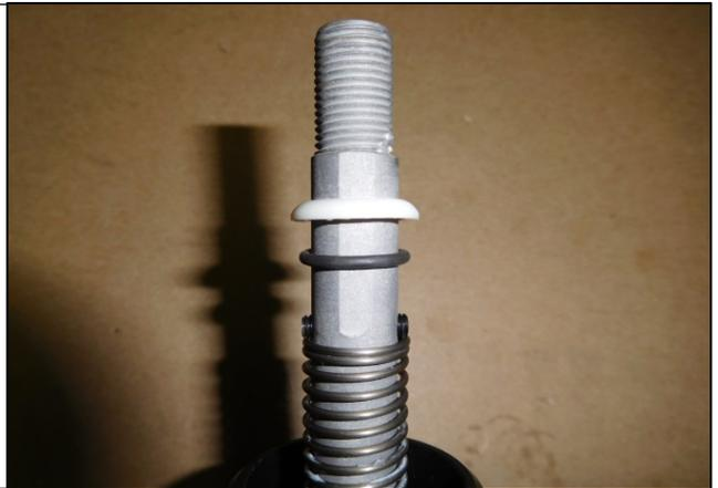
9. Remove the spring retaining roll pin and the spring. The spring will be reused.
