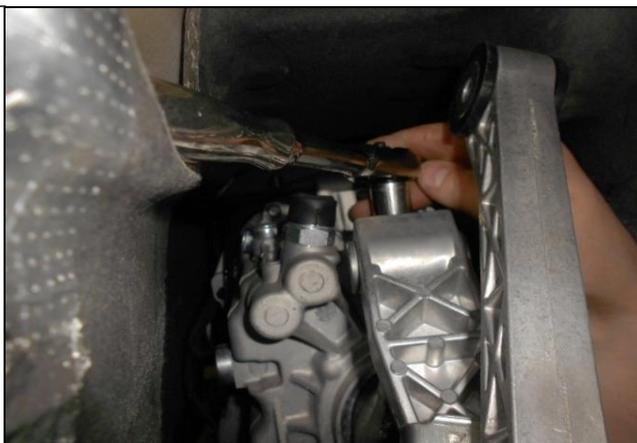
22. The photo to the right is a close up of the bolt removed from the shift linkage. Note that the bolt is only partially threaded at the top. This is being mentioned so you don't spend too much time trying to loosen a bolt that is already completely loose. After it is completely loose, it will need to be pulled free.
