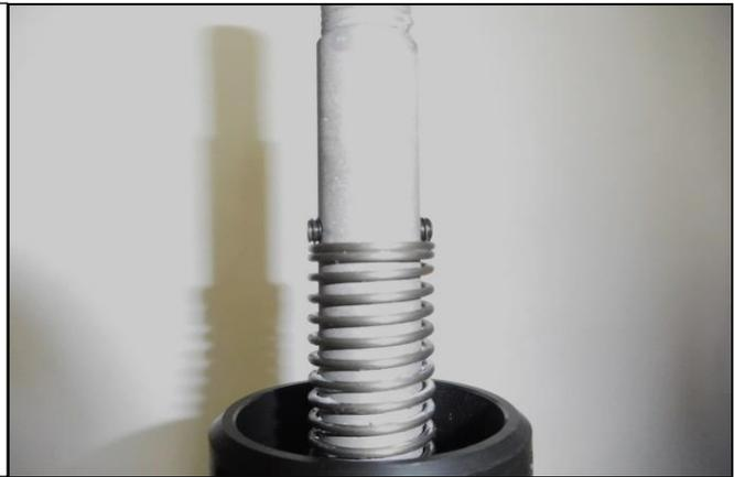
44. Reinstall the O-ring and plastic ring that were removed in step 7.
