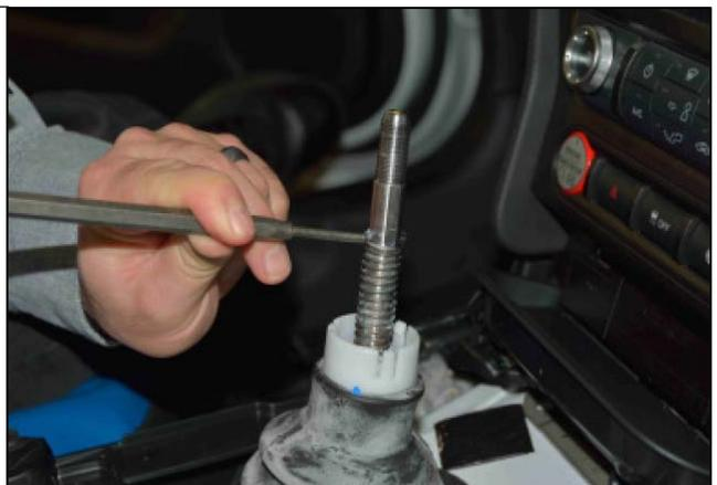
10. Remove the retaining screw and then remove the factory reverse lockout sleeve and rubber boot. The retaining screw and rubber boot will be reused.
