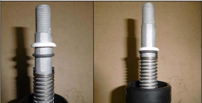
45. Reinstall the rubber boot slide it down over the reverse lockout. Seat the bottom of the boot on the shifter housing. The upper portion of the boot will slide down into the machined groove on the reverse lockout.
