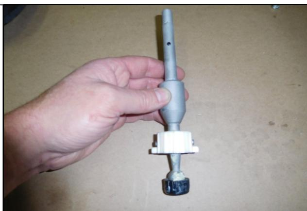
34. Install the Indy shifter into the factory housing. The threaded hole on the large portion of the Indy shifter must be orientated to left side of the shifter housing looking forward.
