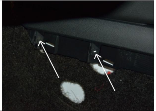
4. Unsnap the shift boot bezel from the console. Lift from the top to release the top clips and then use the pry tool to un-clip the rest.
