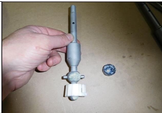
33. Apply the provided grease to the small factory pivot cup and snap it into place on the small ball portion of the Indy shifter stick.
