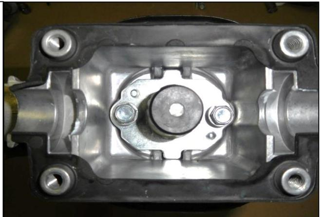
Working in reverse order from step 29 to 24, reinstall the factory shift rod and assemble the shifter housing. Re-torque all bolts to factory torque specifications apply grease to all pivot points.
