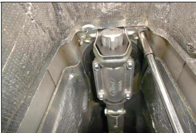
20. Remove the bolt attaching the shifter housing to the transmission.
