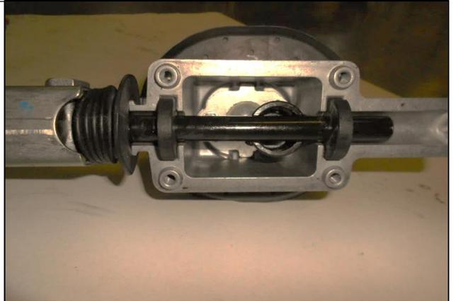
29. Remove the shift rod from the shifter housing.
