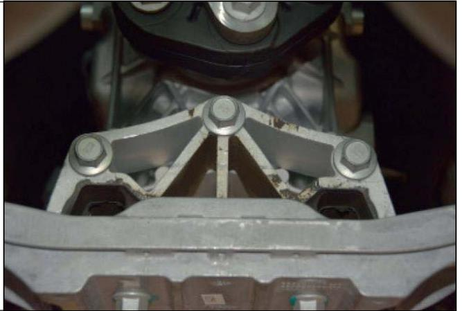
16. Remove the three (3) 18mm bolts securing the front end of the driveshaft to the transmission.
