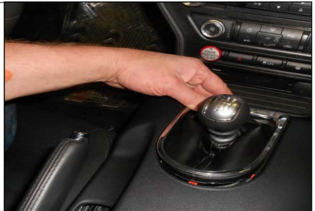
5. Remove the center console. Start by releasing the locking tabs at the rear of the console while working your way forward.
