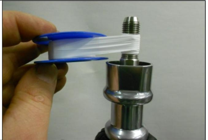
53. Apply the included LOCTITE® 271 thread lock compound to the threaded portion above the Teflon tape.
