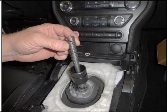
43. Compress the spring enough to install two of the provided set screws. Install the set screws evenly tightening them against each other.
