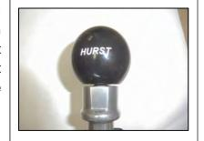
Check for proper operation by engaging the reverse lockout and making sure the shifter will go into reverse.
