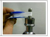
Apply the included LOCTITE® 271 thread lock compound (included) to the threaded portion above the Teflon tape.
