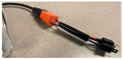
Example shown of what a completed 4652/4656 harness will look like. Not all vehicles will match this diagram. It is imperative that the vehicle harness is checked to ensure wires are matched properly before powering on.
