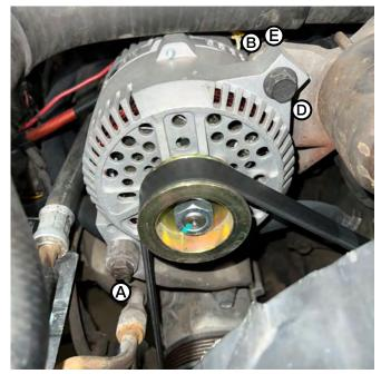
Upper Bolt Washer (B) is located between the nut and bracket.
