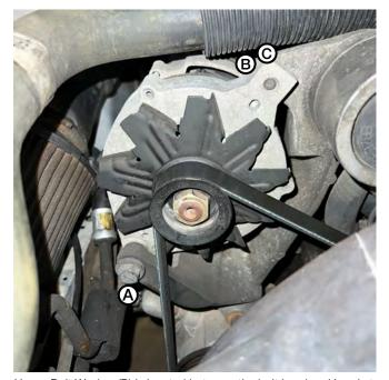
Upper Bolt Washer (B) is located between the bolt head and bracket.
