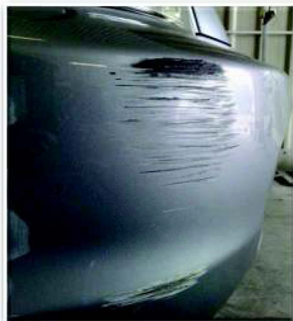
Paint is rubbed off due to impact Not warrantable
