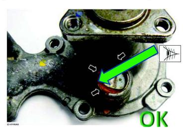
Staining on the pump indicates an earlier event or normal operation which does not constitute as a water pump failure. Slight staining and residual dried coolant build up around the weep chamber vent is considered normal
