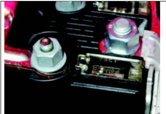
Figure 4: Example High Amp Fuse at High Current Battery Junction Box on 2014 F150.
