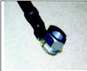
Figure 1: Example Threaded Connector at High Current Battery Junction Box 2014 Escape
