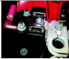
Figure 2: Example eyelet type connector at High Current Battery Junction Box 2014 F150
