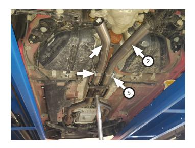
9. Place clamps (x2) (5) onto left and right muffler assemblies (3, 4) and connect them to mid pipes. Rebolt hanger mounts (x4) onto frame and press hangers into mounts as shown.
