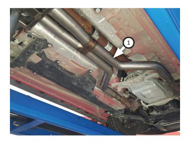
8. Place clamps (x2) (5) onto right and left mid pipes (2) and connect them to scavenger outlets. Tighten clamps enough to allow for adjustment.
