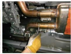
4. Unbolt hangers (x2) behind rear differential. Then carefully slide exhaust system forward and out of rear hanger mounts and lower system to floor. Finally, remove hanger mounts (x2) from rear of vehicle.
