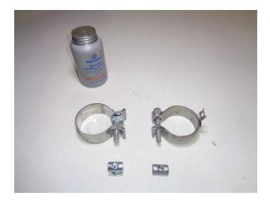
7. Place factory clamps (x2) onto downpipes then connect scavenger (1). Center clamps over connection then tighten them enough to allow for adjustment.
