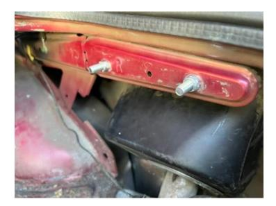
Now that the bolts/studs have been fastened to the body of the car, we reinstall interior side panels and mount the FFP customs Trunk mounts to the studs using the acorn nuts, take care when tightening these bolts to prevent scratches. Orientation of the mounts can be seen in the picture below and is engraved on the back of the mounts (pivot ball should be towards the front of the car).
