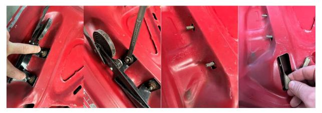
Once, the stud plate is out rotate it 180\*. Now with the studs facing the center of the trunk lid, slide the provided U-nut over the hole that is closest to the back of the trunk lid. Now guide the stud plate back into the hole that it was removed from and line up the U-nut to the factory hole closest to the back of the trunk lid.
