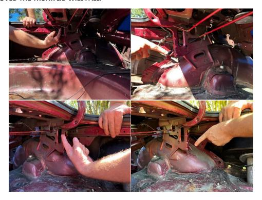
Once the torsion springs are removed, if you are running interior side panels now is the time to mark the holes and drill to a 9/16" hole for the mounting studs and hex nut to pass through (we like to use a step bit). The pictures below show both factory holes used to mount the trunk mounts as well as the holes drilled in the interior side panels.
