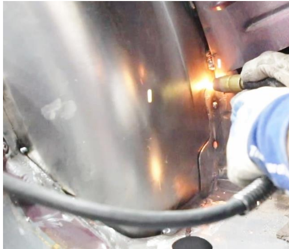
Figure 39 - Tack Weld Flange
