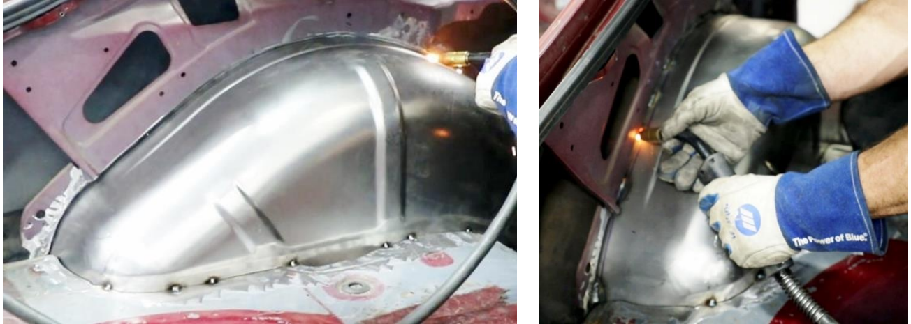
Figure 38 - Tack Weld Mini-Tub
