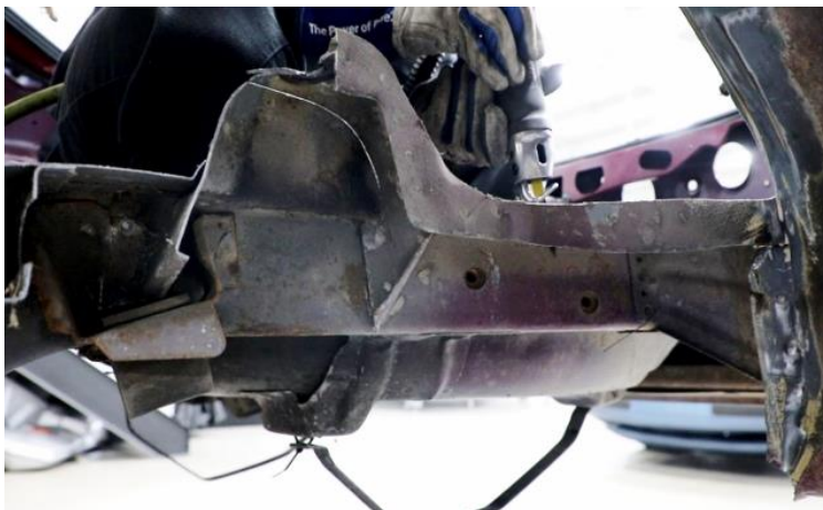
Figure 20 – Remove Rear Factory Structure
