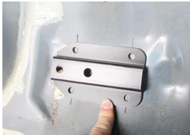
Figure 45 - Transfer Punch Holes
