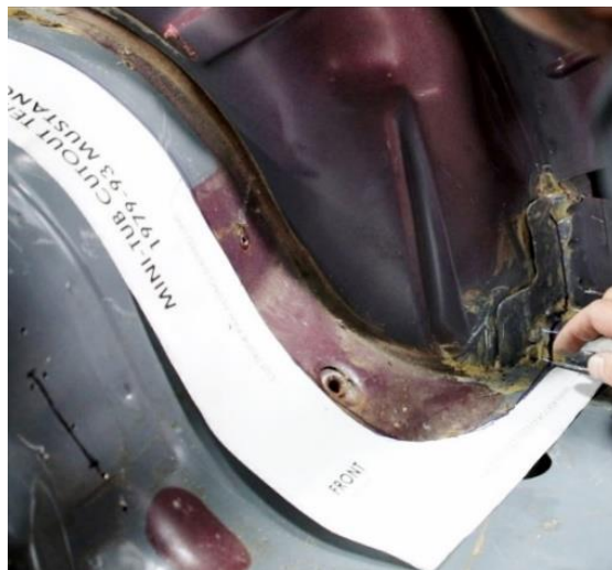
Figure 15 – Locate Front Template
