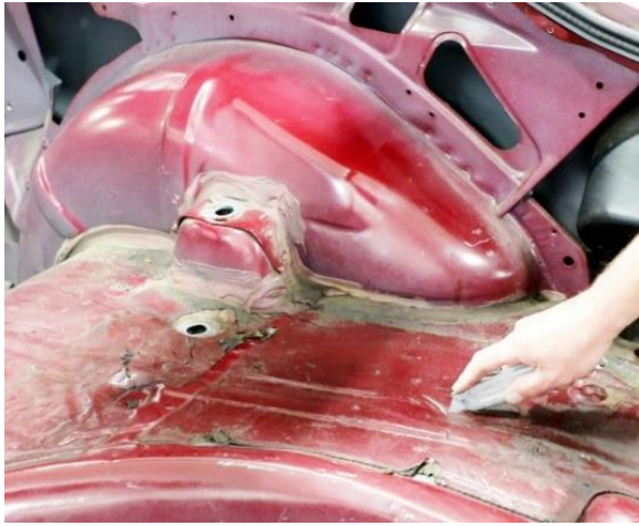
Figure 4 - Remove Trunk Pan Material
