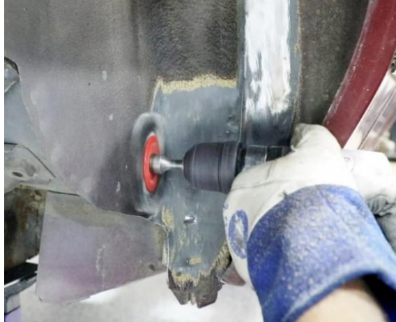
Figure 10 - Locate Spot Welds
