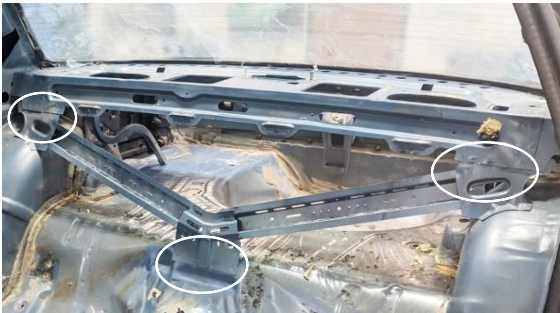
Figure 3 - Remove Wheel Tub Brackets
