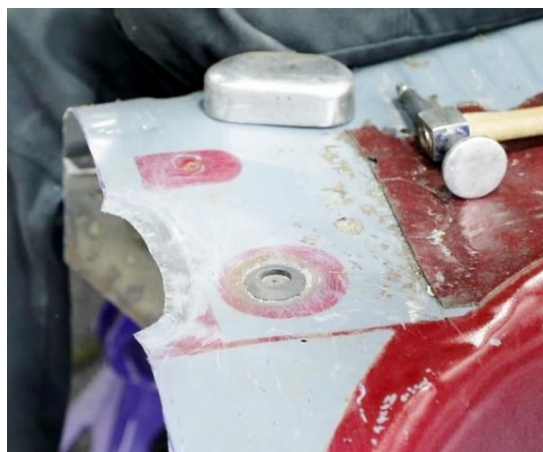
Figure 29 - Flatten Trunk Floor
