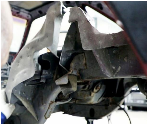
Figure 19 – Remove Front Factory Structure
