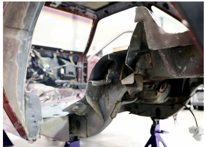
Figure 19 – Remove Front Factory Structure
