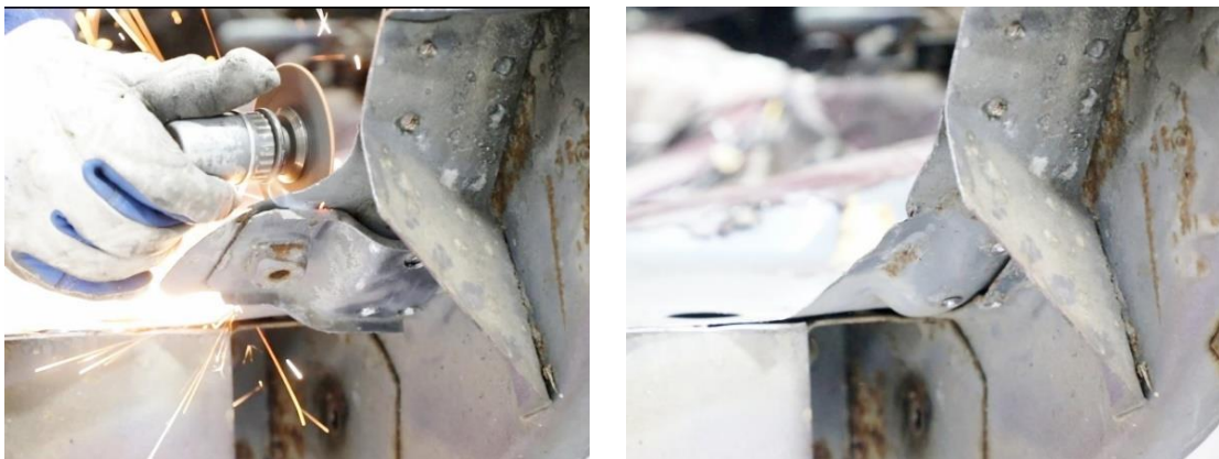
Figure 28 - Remove Seat Belt Anchor
