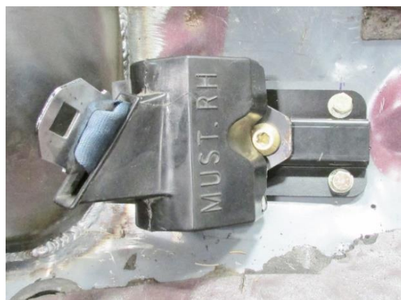
Figure 49 - Torque Seat Belt Assembly
