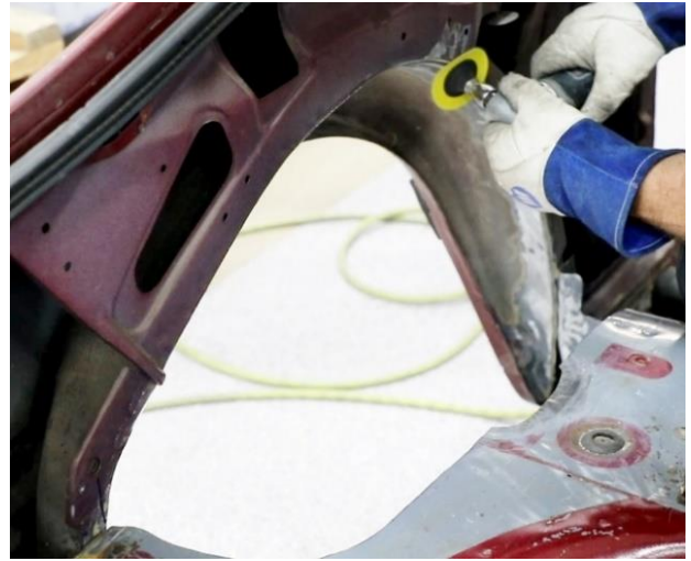
Figure 32 – Grind Sheet Metal
