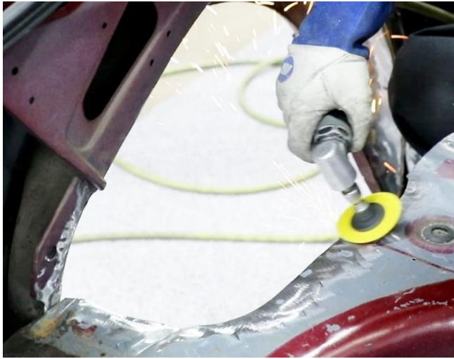
Figure 32 – Grind Sheet Metal
