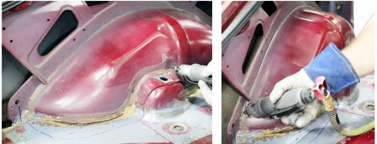
Figure 17 - Cutout Inner Wheel Tub
