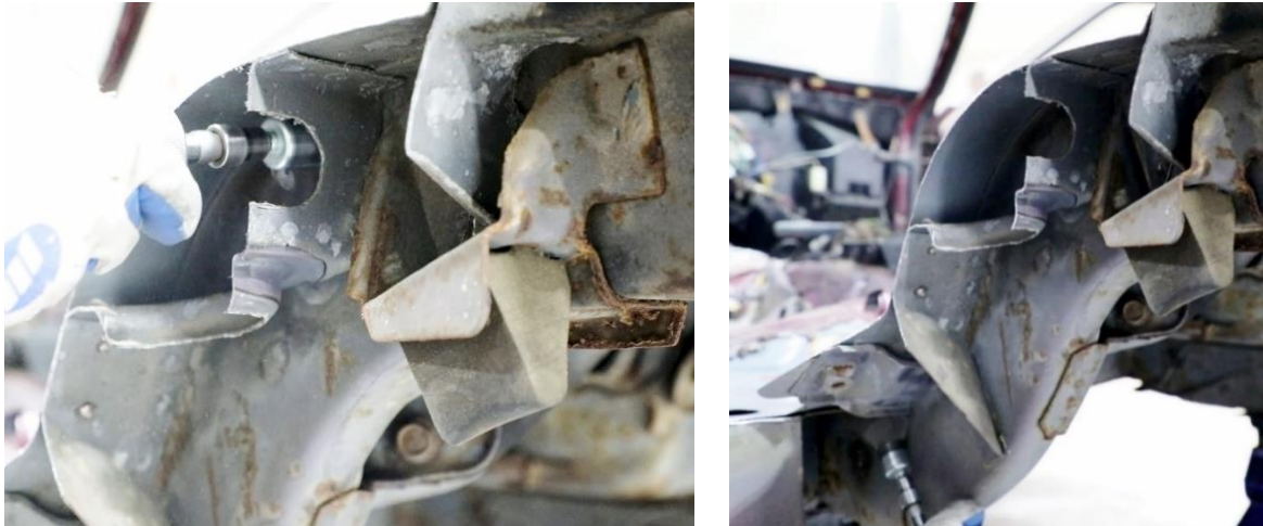
Figure 22 - Expose Spot Welds
