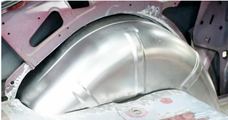
Figure 33 – Test Fit Mini-Tub
