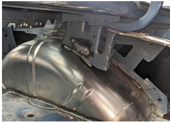
Figure 50 - Re-attach Trunk Hinge Bracket
