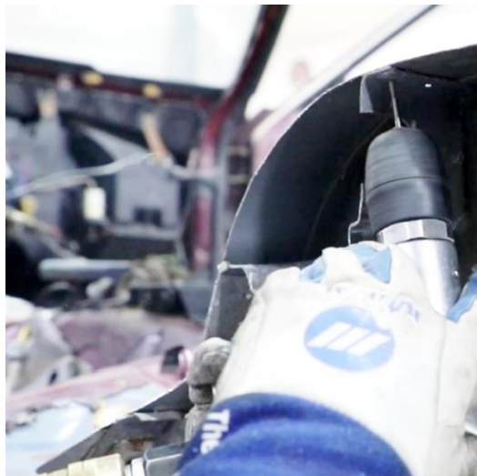
Figure 26 - Remove Spring Perch Spot Welds
