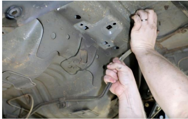
Figure 21 - Bend Fuel Lines
