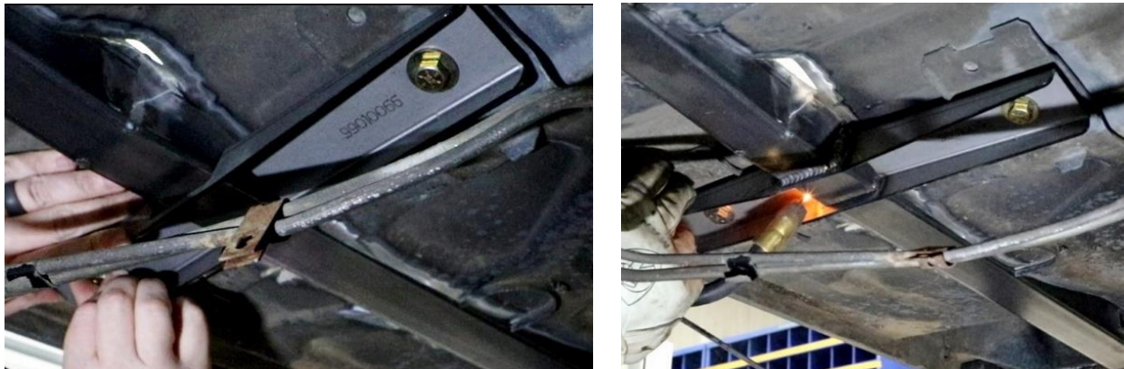
Figure 55 – Install Seat Mount
