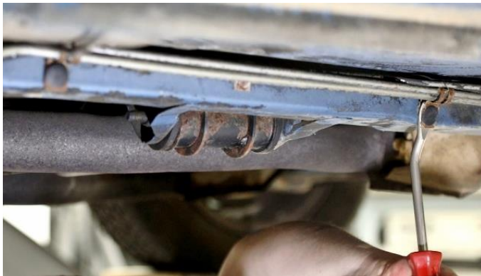
Figure 2 – Remove Fuel & Brake Line Clips
