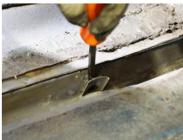
Figure 17 – Remove Floor Pan Bracket
