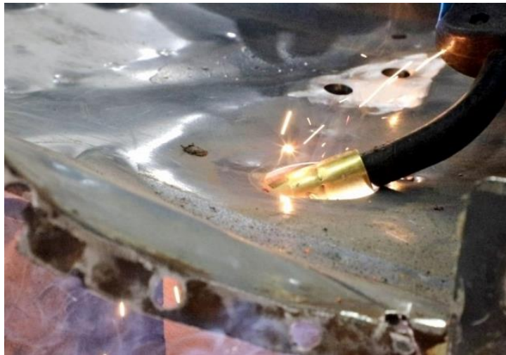
Figure 49 – Tack Weld Torque Box
