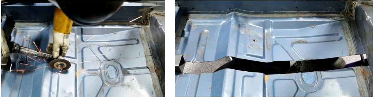
Figure 25 – Cut Floor Pan
