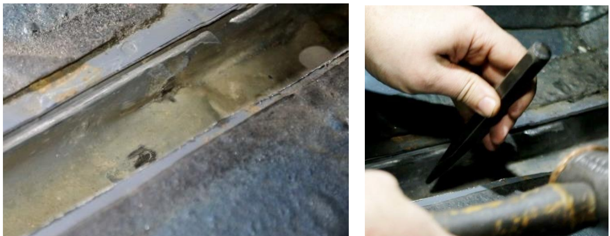
Figure 21 – Grind Away Burrs
