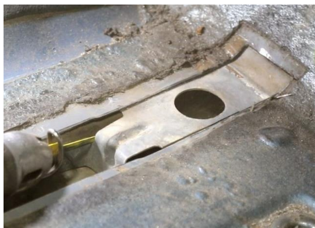
Figure 17 – Remove Floor Pan Bracket
