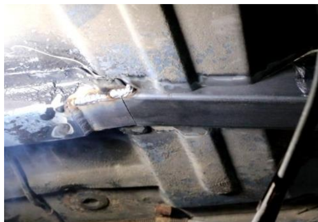
Figure 47 - Weld Sides of Connector
