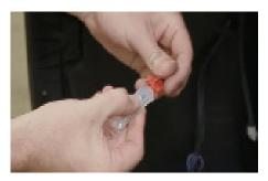
**10.** In order to properly connect the wires and ensure protection against moisture, take a red electrical connector, open it, and squeeze a small amount of the included dielectric grease into the connector, directly in the middle.
