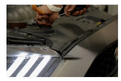
**1.** To begin, using a plastic rivet removal tool or small flathead screwdriver, remove the 8 plastic rivets holding the fascia to the bumper. Set fascia aside.
