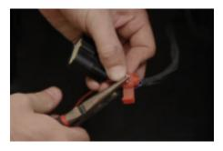
**13.** Verify that the inner pigtail wire is fully inserted on the inner groove, and the vehicle wire is aligned straight through the outer groove. Then, use pliers to clamp down the metal splice. Check to be sure the connection is secure after splicing by slightly tugging the wires, then clip the connector cover closed Repeat for each wire on both sides.
