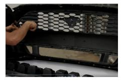
**6.** Next, remove the factory grille by depressing the clips using a flathead screwdriver.
