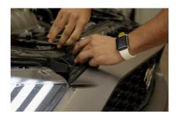
2. Using an 8mm socket, remove the 6 screws from the top of the bumper. Then remove the two 5.5mm screws at the top corners of the fascia near the headlight, under the weather strip. Then using a 7mm socket, remove the 12 screws from underneath the bumper.
