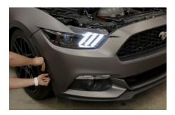
**3.** Using a plastic rivet removal tool or small flathead screwdriver, remove the 2 plastic rivets holding the bumper to the wheel well. Then remove the 7mm bolt that retains the fender to the fascia on both sides. Pop out the locking clips at the top corner of the bumper, and repeat for the other side of the vehicle.
