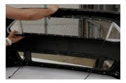
**7.** Install your Classic Design Concepts Outlaw Switchback Grille by snapping the clips into place. Then reinstall the backing back onto the bumper assembly.
