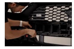
**5.** Looking at the rear of the bumper assembly, remove the lower backing piece by depressing the 6 clips using a flat head screwdriver. Set the backing aside.
