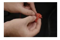
**11.** Squeeze the connector slightly back together. You will notice that the connector has two grooves. On the inner groove of the connector, one side is blocked. Slide the end of one of the pigtail wires into this inner groove of the connector. Be sure to hold this wire all the way in the connector until it is secured.
