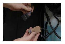
8. Unplug the factory headlamp connectors by reaching up and behind each headlamp, and depressing the clip on the connector. Identify the brown turn signal connectors on each side. On each connector, remove 2-4 inches of wrapped insulation in order to access wires.
