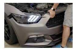
**4.** Remove the bumper by pulling straight off, evenly on both sides. Make sure the clips at the top of the wheel well are unclipped. Unplug any wiring, including bulbs and sockets, and set the bumper on a soft surface.
