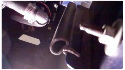
Raise FILTER up onto the JLT tube. By TWISTING the tube at the throttle body you can gain more room right or left. I/C hoses can and will touch the filter, just make sure there is not hard pressure on the filter causing the hose to kink.
