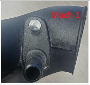
**8** Attach reducer and clamps to the small end of the JLT tube and the air filter to the large end. Lower tube assembly down onto throttle body and into airbox.
