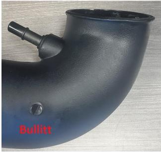
**Mach I:** You will install the fitting assembly into the hole on the underside of the intake tube and plug the hole near the PCV fitting with the supplied 3/8's plug.
