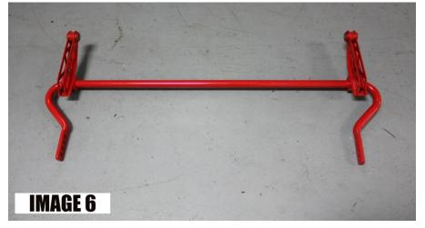
Energy Suspension bushings, connect the BMR end links to the BMR sway bar as shown in **IMAGE 6**. Use the provided 3/8" Allen bolts, nuts, and washers for this connection.
