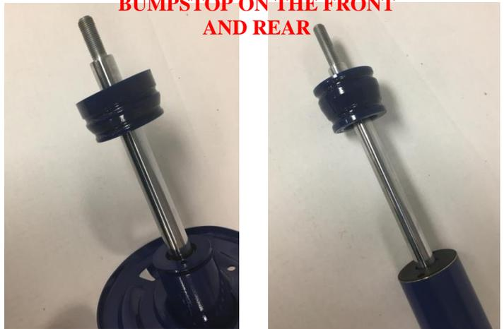
**Use the provided o-rings on the REAR shocks below the bumpstops for lowered applications**
