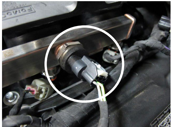
Fig. 5-e: Disconnect Fuel Rail Pressure Sensor
