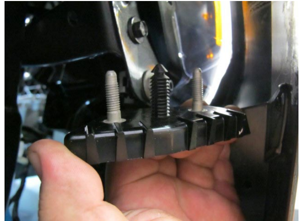
Fig. 1-j: Remove Corner Brackets
