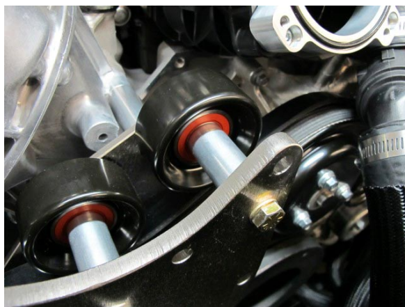
Fig. 2-m: Install Previously Removed Smooth Idler Pulley
