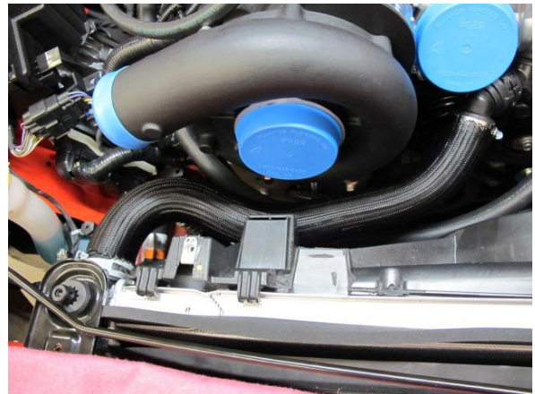
Fig. 3-d: Upper Radiator Hose (New Configuration)
