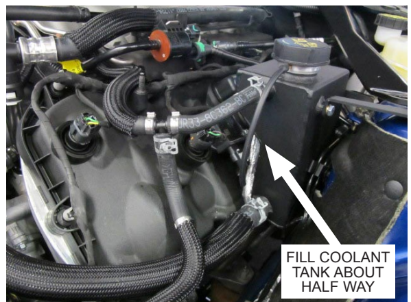
Fig. 3-q: Refill Cooling System
