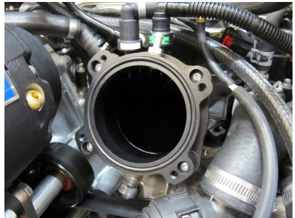
Fig. 4-b: Install Throttle Body Spacer
