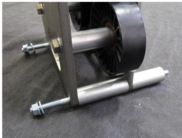
Fig. 2-h: Keep 2x 2.730" Spacers In Place
