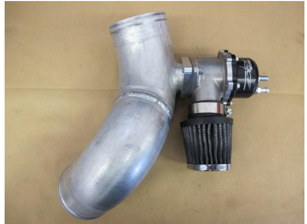
Fig. 4-an: Install Bypass Valve
