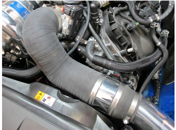
Fig. 4-aw: Secure All Hose Clamps
