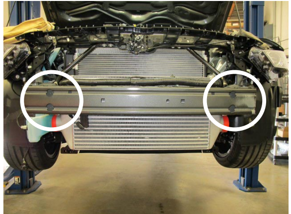
Fig. 4-af: Charge Air Cooler Installation
