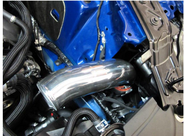
Fig. 4-at: Install Discharge Tube D
