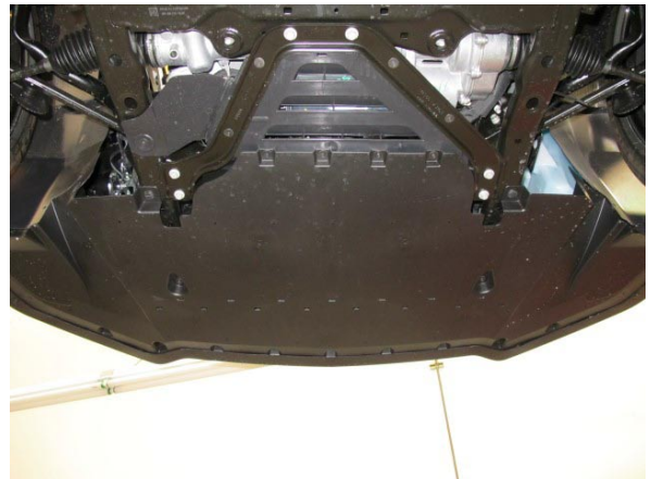
Fig. 1-k: Remove Lower Splash Guards
