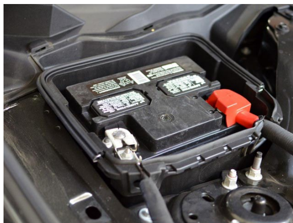
Fig. 1-b: Unplug Battery Leads
