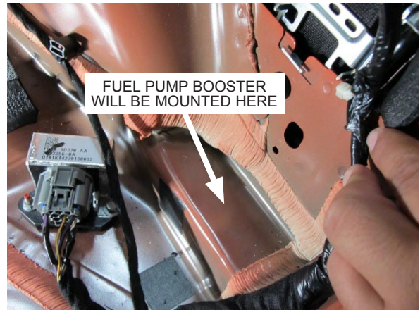
Fig. 6-j: Fuel Pump Booster Mounting Location
