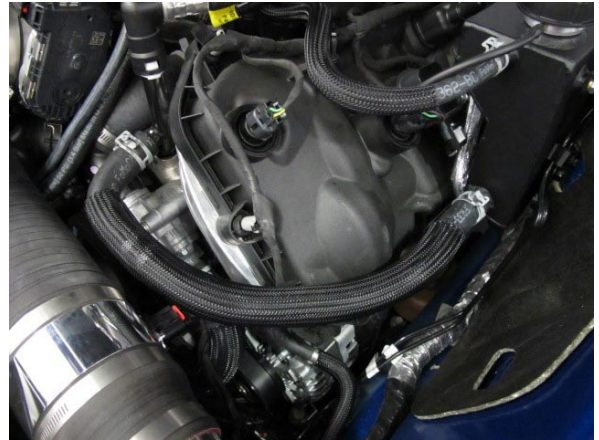
Fig. 3-p: Secure Modified OEM 3/4" Coolant Hose
