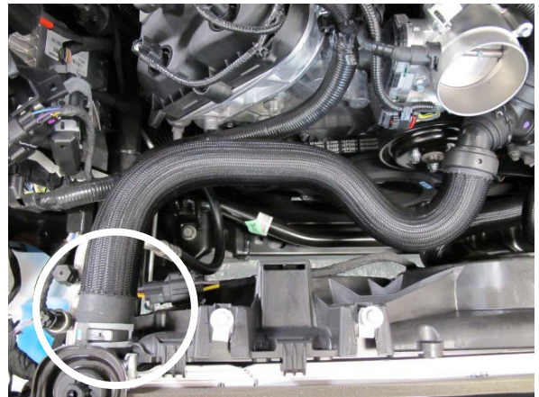
Fig. 3-b: Upper Radiator Hose (OEM Configuration)
