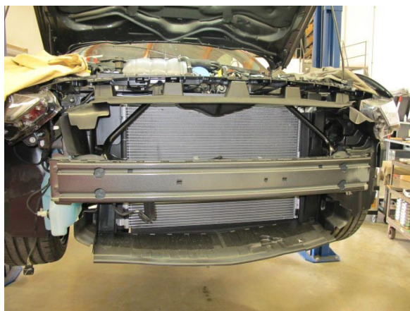
Fig. 1-m: Remove Front Bumper Cover
