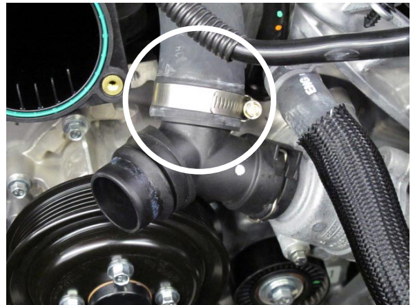
Fig. 3-a: Install #24 Hose Clamp
