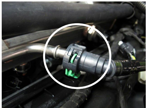
Fig. 5-f: Disconnect Low Pressure Fuel Feed Line
