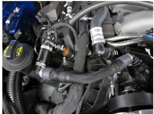
Fig. 7-e: Install PCV Assembly
