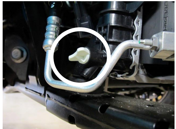
Fig. 1-q: Drain Engine Coolant
