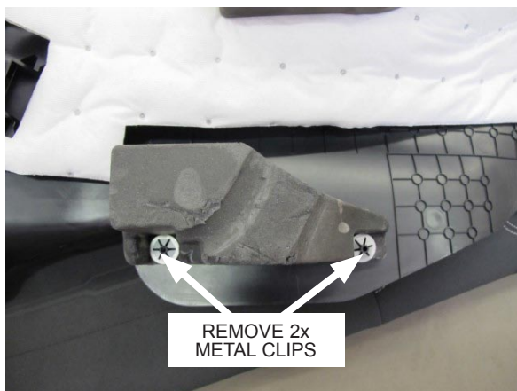
Fig. 6-i: Remove Foam Insulation Block
