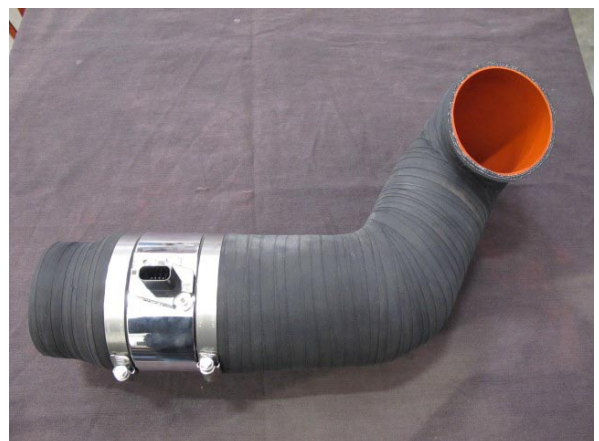
Fig. 4-av: Assemble MAF Sensor Housing & Sleeves As Shown
