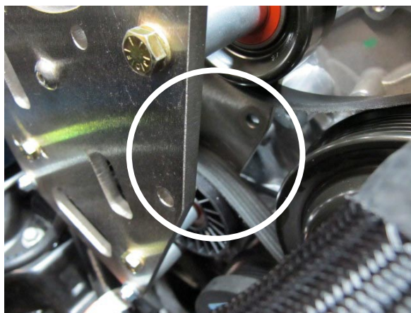
Fig. 2-n: Remove This 1x 2.730" Spacer & Set Aside
