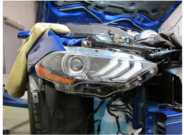
Fig. 1-w: Remove Passenger Side Headlight
