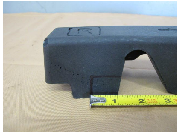
Fig. 5-m: Modify Passenger Side Fuel Rail Cover
