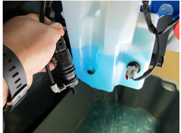
Fig. 4-d: Drain Windshield Washer Fluid Reservoir
