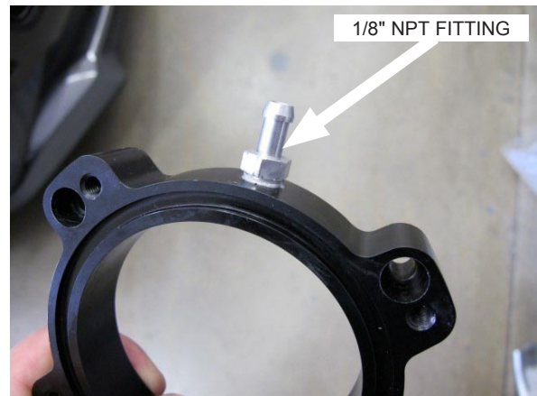
Fig. 4-a: Install 1/8" NPT Fitting
