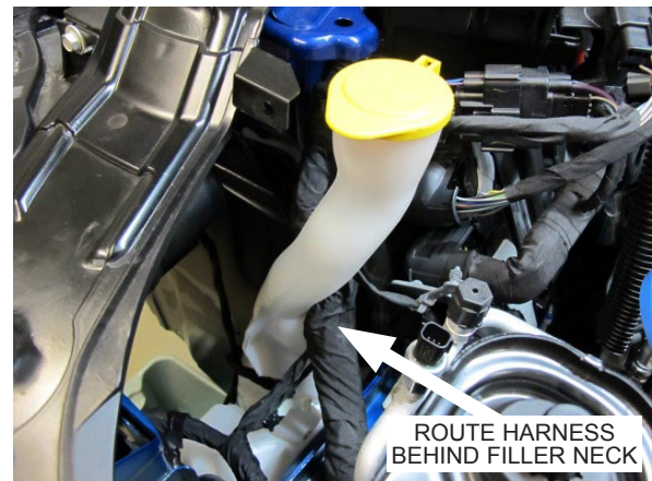
Fig. 4-k: Reinstall Windshield Washer Fluid Reservoir
