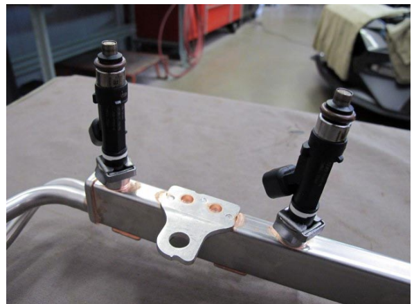
Fig. 5-i: Make Note Of Fuel Injector Orientation
