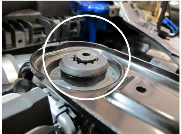
Fig. 7-n: Modify Radiator Mounting Tabs
