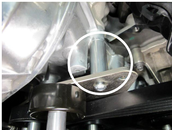
Fig. 2-j: Install 1x 2.058" Spacer
