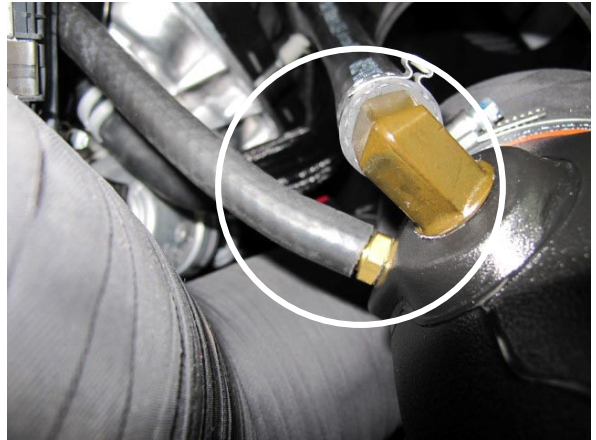
Fig. 7-m: Install 3/8" Hose, Then Secure Air Inlet Tube
