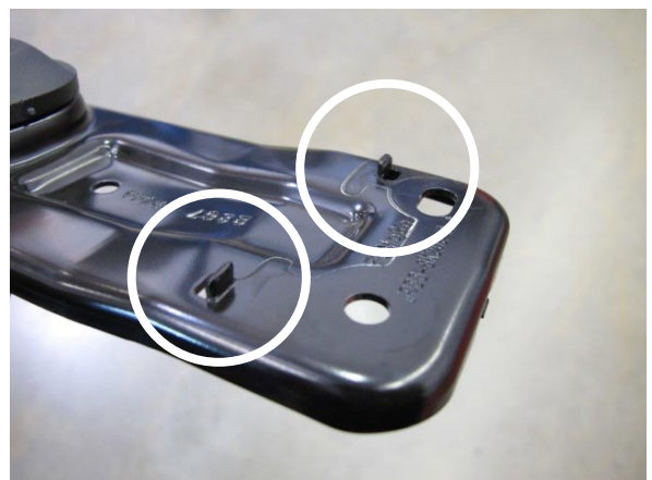
Fig. 4-o: Remove 2x Protruding Tabs
