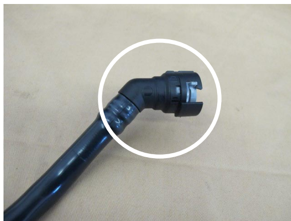
Fig. 7-b: Remove 45° Quick-Release Fitting
