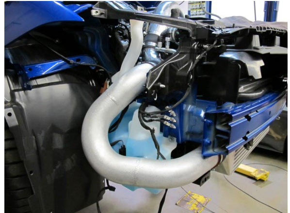
Fig. 4-aq: Install Discharge Tube B
