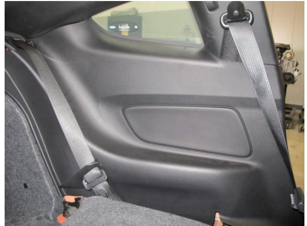
Fig. 6-p: Reinstall Driver Side Rear Interior Panel
