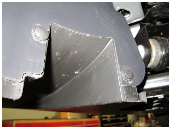
Fig. 1-g: Remove Plastic Fasteners
