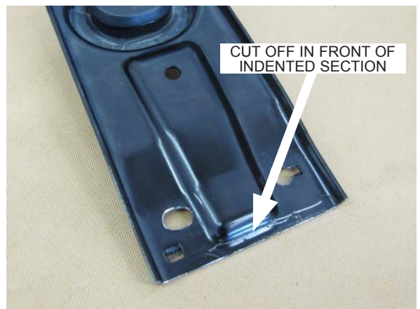
Fig. 4-r: Cut The Upper Radiator Bracket As Shown
