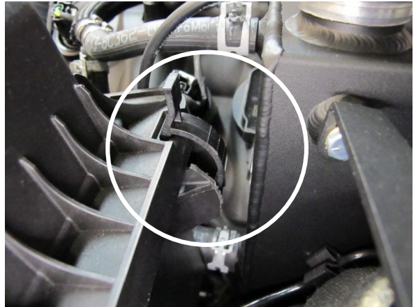
Fig. 7-g: Trim Air Box As Necessary
