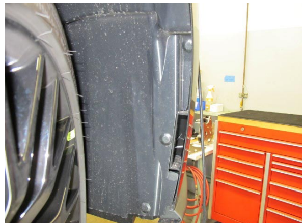
Fig. 1-f: Remove Fender Liner Fasteners
