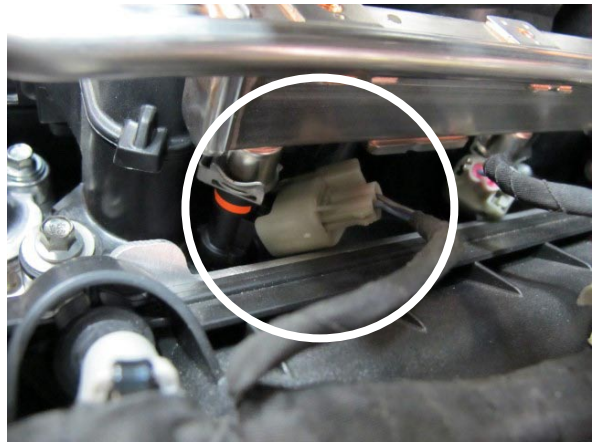
Fig. 5-d: Disconnect Fuel Injectors
