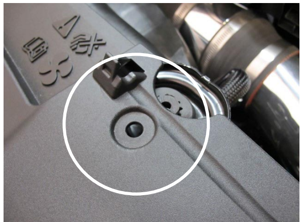
Fig. 7-o: Check Upper Radiator Support Cover
