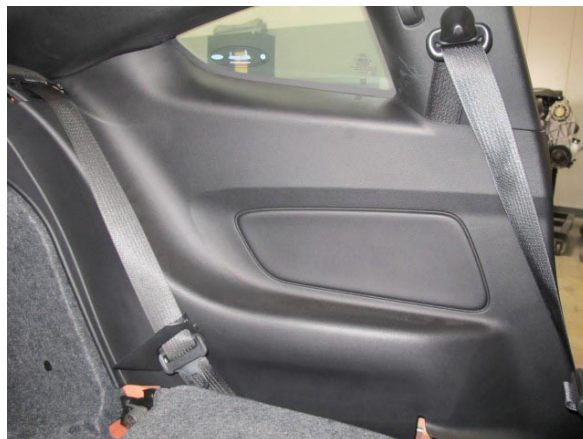
Fig. 6-g: Remove Driver Side Rear Interior Panel
