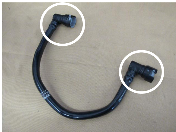
Fig. 7-a: Remove Both Quick-Release Fittings
