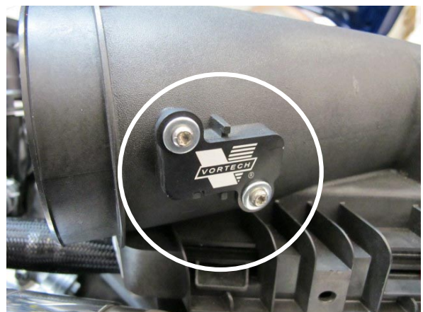
Fig. 7-f: Install MAF Block-Off Plate
