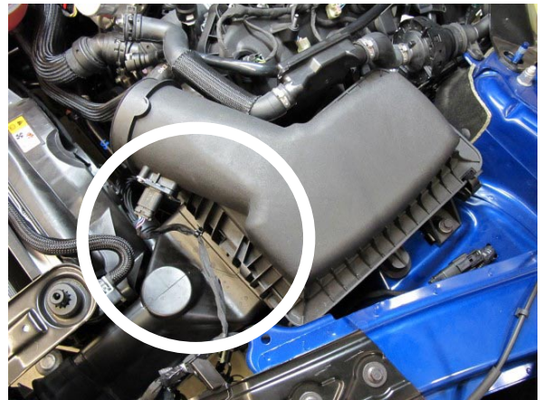
Fig. 1-p: Remove Air Box
