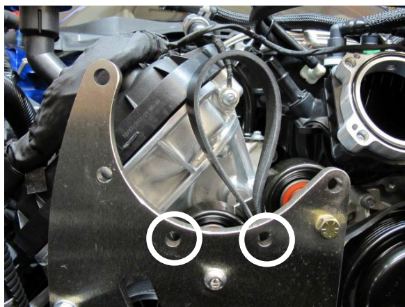
Fig. 2-o: Use long 9/16" Wrench To Install These Screws
