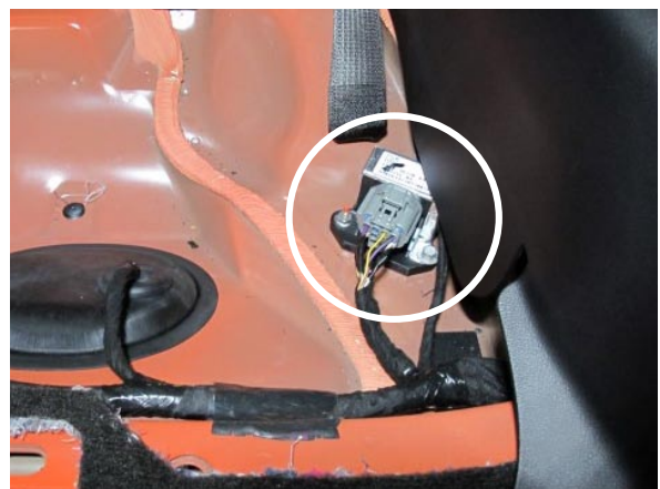
Fig. 6-c: Unplug Fuel Pump Driver Module
