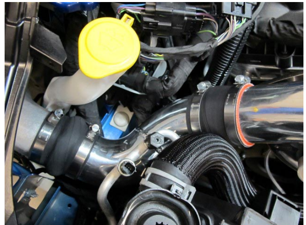
Fig. 4-ao: Install Discharge Tube A
