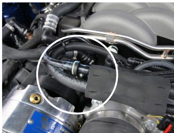
Fig. 7-k: Install 24" Length Of 3/8" Hose
