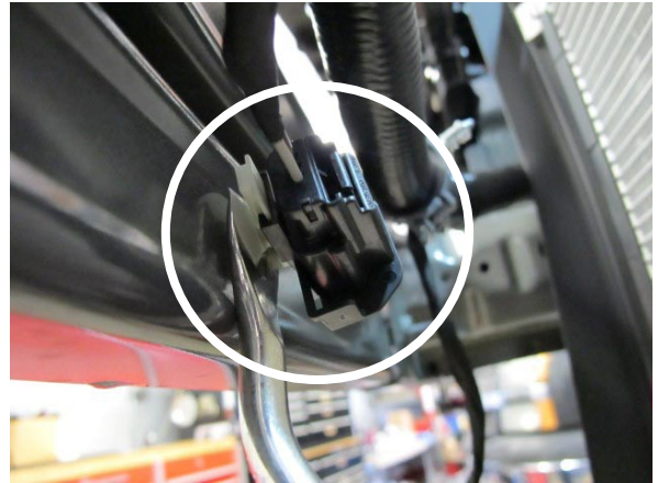
Fig. 4-v: Remove Unused Plug From Front Bumper Support
