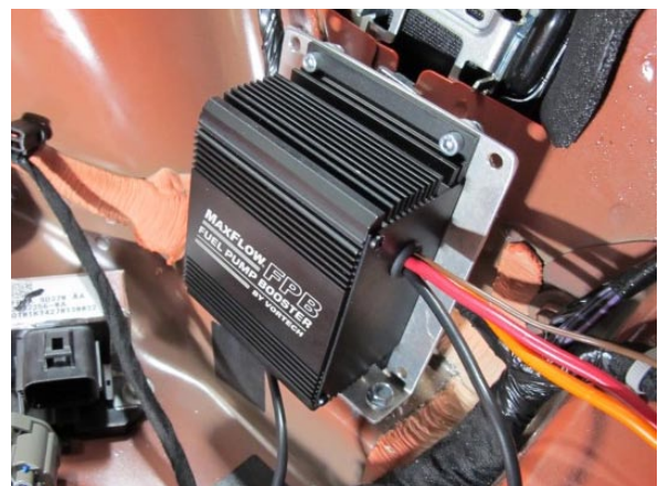
Fig. 6-l: Mount Fuel Pump Booster
