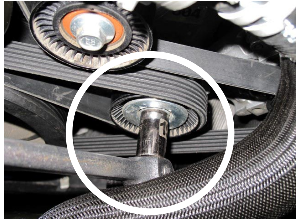
Fig. 2-s: Install Supercharger Drive Belt
