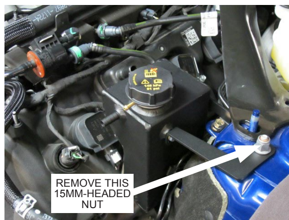
Fig. 3-k: Loosely Attach Coolant Tank
