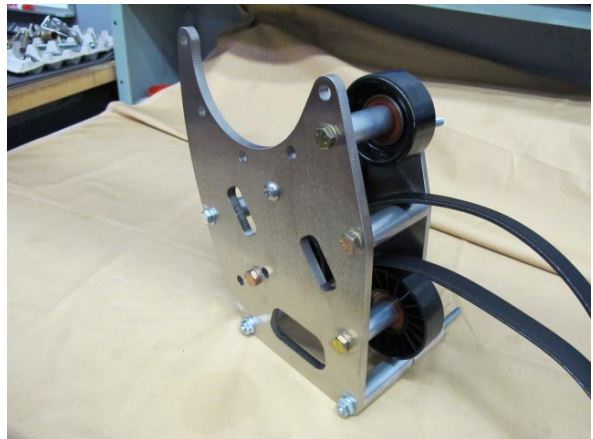
Fig. 2-b: Inspect Supercharger Mounting Bracket Assembly
