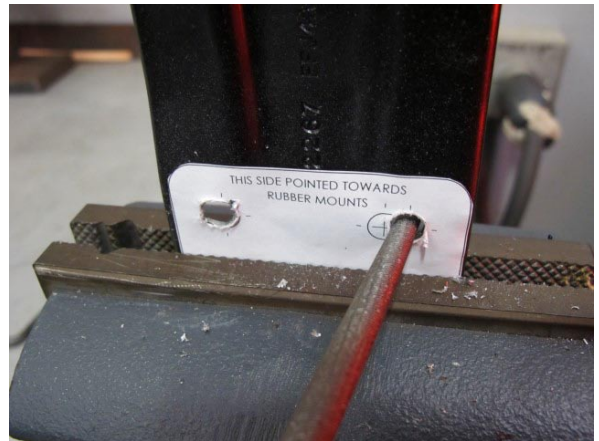
Fig. 4-q: Use Round File To Slot Hole
