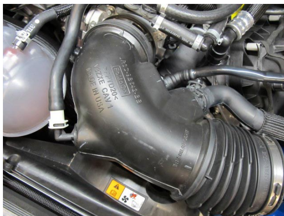
Fig. 1-o: Remove OEM Air Inlet
