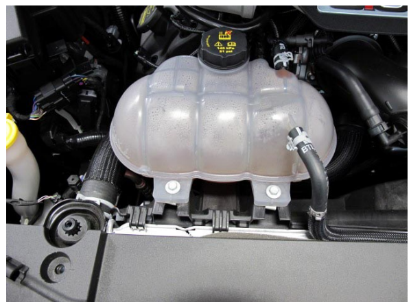
Fig. 1-r: Remove Coolant Reservoir
