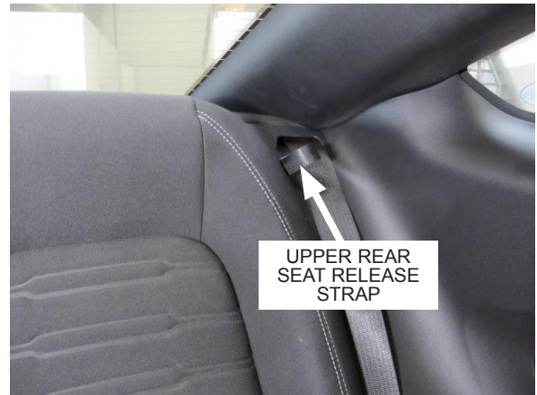
Fig. 6-d: Fold Upper Rear Seat Down
