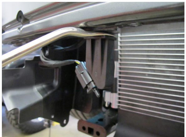
Fig. 4-u: Remove Ambient Air Temperature Sensor
