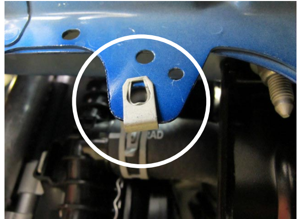
Fig. 4-az: Relocate OEM Threaded Clip
