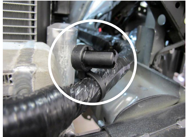
Fig. 4-y: Remove Plastic Harness Clip
