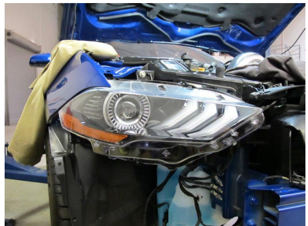
Fig. 4-bb: Reinstall Passenger Side Headlight
