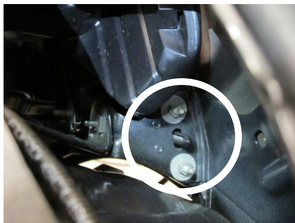
Fig. 1-i: Remove Corner Bracket Fasteners
