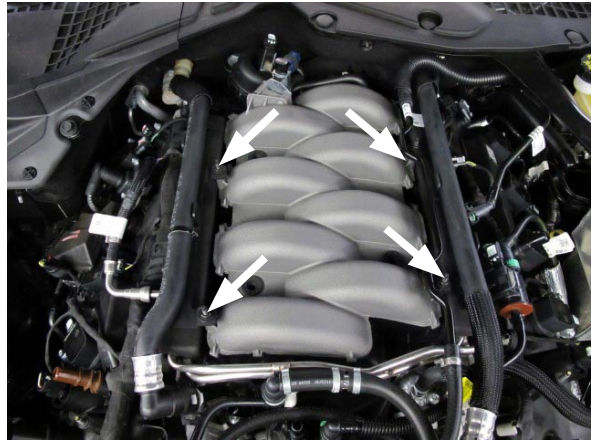
Fig. 5-a: Remove Fuel Injector Rail Fasteners
