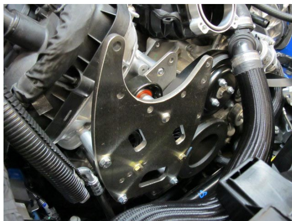
Fig. 2-i: Install Supercharger Mounting Bracket Assembly
