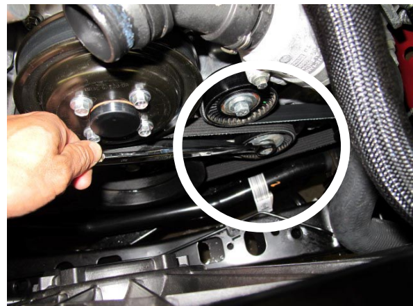
Fig. 1-t: Remove Accessory Drive Belt
