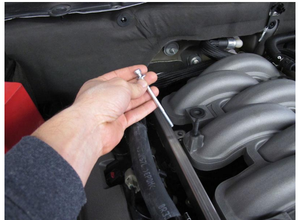
Fig. 5-h: Remove Fuel Rail Assembly
