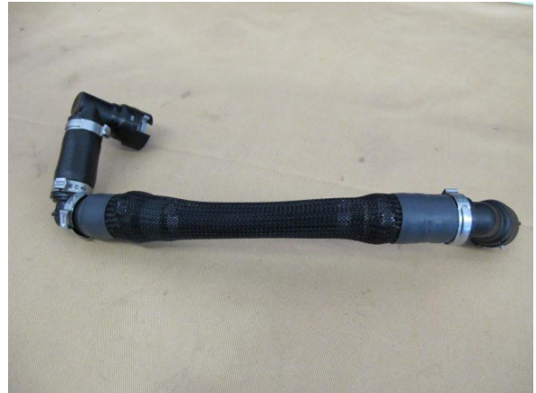
Fig. 7-d: Loosely Assemble OEM Quick-Release Fittings As Shown
