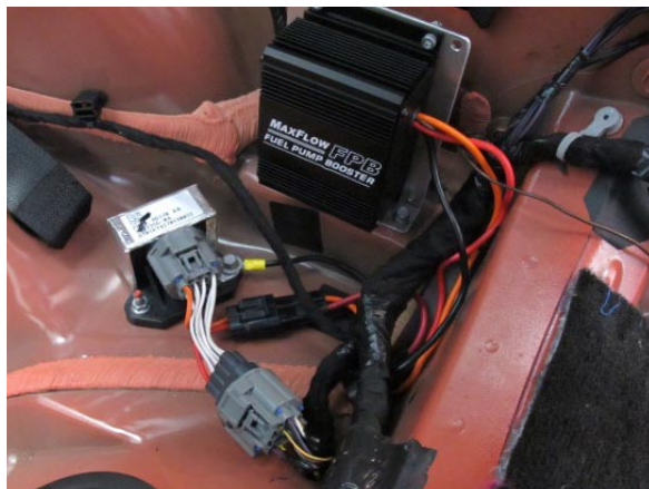
Fig. 6-m: Install Adapter Harness
