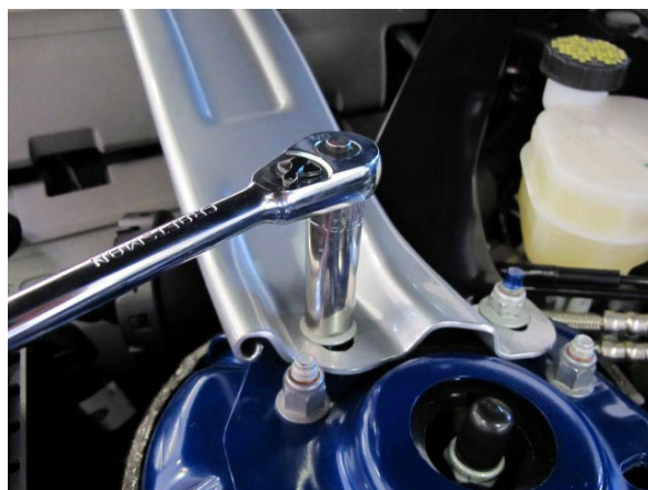
Fig. 1-c: Remove Strut Tower Brace
