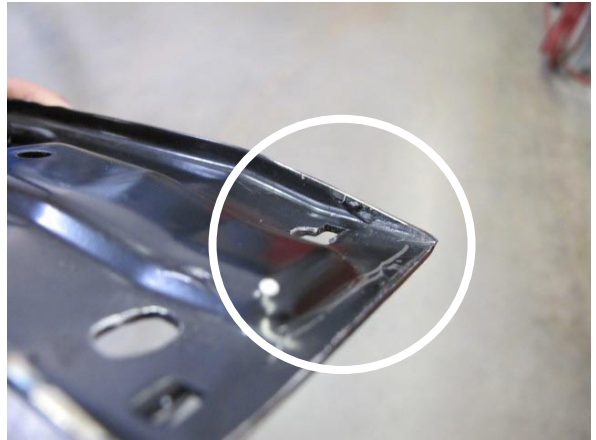
Fig. 4-s: Grind Down Raised Edges To A Taper
