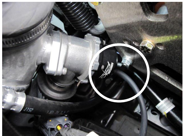
Fig. 4-ay: Attach Vacuum Hose To Bypass Valve
