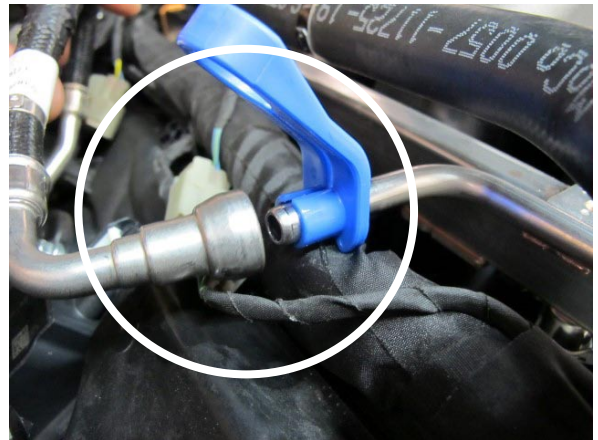
Fig. 5-g: Disconnect Direct Injection Fuel Line
