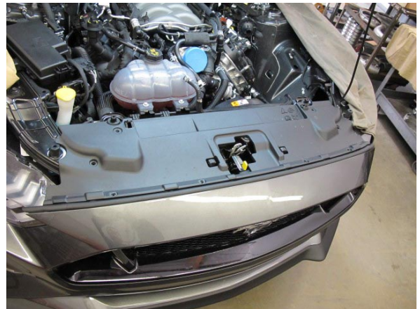
Fig. 1-d: Remove Radiator Support Cover
