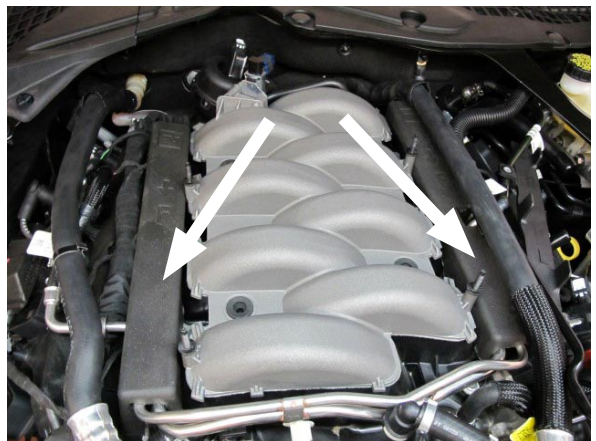
Fig. 5-c: Remove Fuel Injector Foam Insulation
