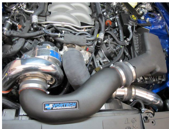
Fig. 7-l: Loosely Install Air Inlet Tube
