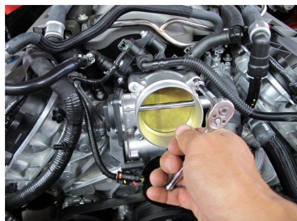
Fig. 1-u: Remove Throttle Body
