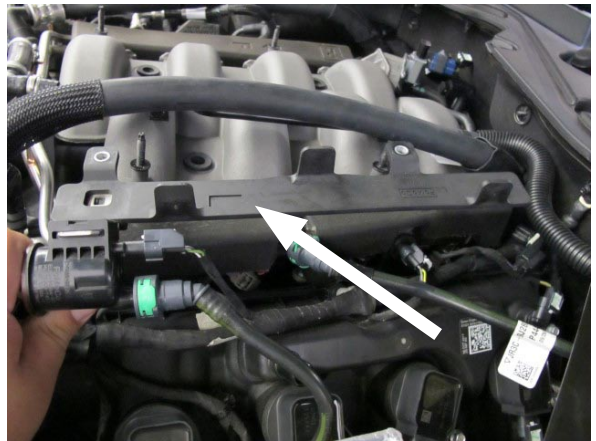
Fig. 5-b: Set Driver Side Heater Hose Guide Aside
