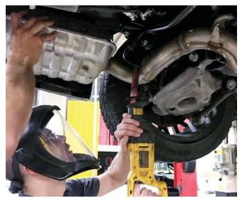
3. With the exhaust pipe cut, slide the hanger out of the rubber mount and remove the muffler/tip assembly from the vehicle.
