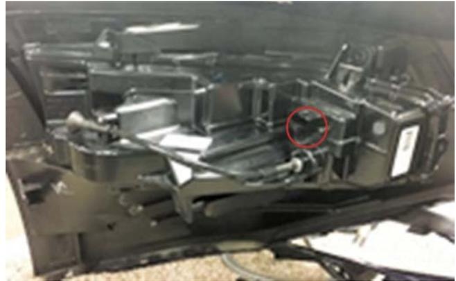
7. Remove the two (2) nuts and one (1) push pin holding the fascia to the fender. Repeat on the other side of the vehicle.
