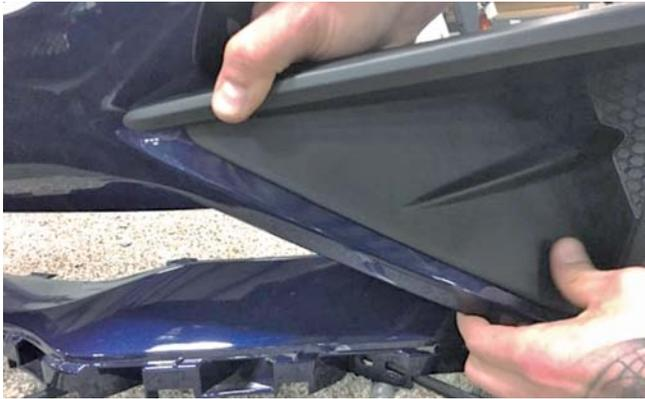
13. Hand start the M5 bolt (PN: 9809A316) to the back of the bracket. Repeat on the other side of the fascia.
