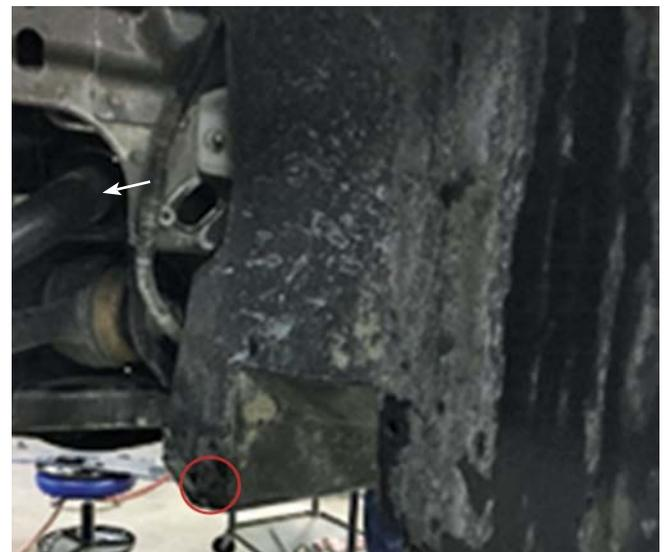
3. Remove the five (5) push pins and remove the fender liner as shown. Repeat on the other side of the vehicle.
