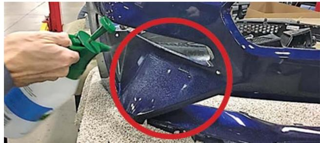
11. Rewet the surface with soapy water and apply graphic (PN: 1318-17B671RH or 1318-17B671LH) to wet area. Use a flexible plastic squeegee to apply graphic and work all bubbles to outer perimeter. Repeat on the other side of the fascia.
