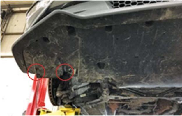
5. Remove the seventeen (17) (nineteen [19] for performance package) 8 mm screws from the undertray. Remove the two (2) push pins and remove undertray from the vehicle.
