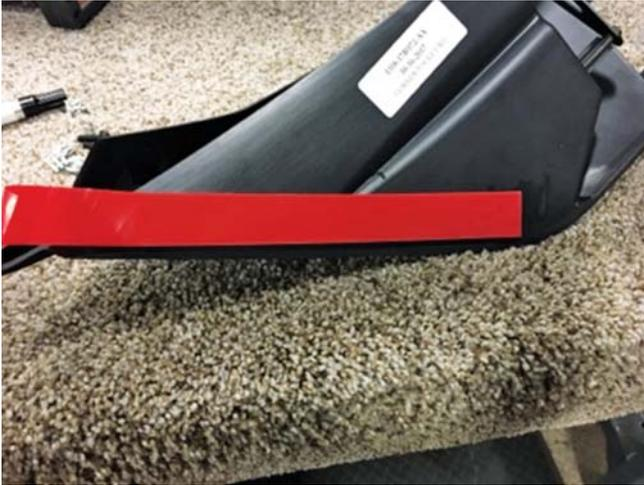
9. Fasten bracket (PN: 1318-17C974 for right-hand side or 1318-17C973 for left-hand side) to the three (3) plastic studs using three (3) of the supplied M4.2 screws (PN: 12741) and a 7 mm socket. Torque to 2 Nm. Repeat on the other side of the fascia.
