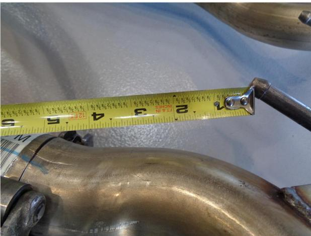
**Step 1.** Begin removing the OEM exhaust system by cutting both pipes exiting the resonator. Measure and cut on the driver side 5" from the tip of the hanger. Cut the passenger side also from the tip of the hanger 5.5" back. Next, extract the hangers from the rubber insulators and remove the OEM mufflers. Retain insulators as they will be used to install the new system.
