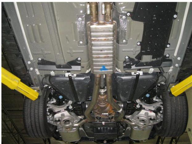
**Step 1.** Begin removing the OEM exhaust system by loosening the clamps located in front of the resonator. Next working front to rear extract the hangers from the rubber insulators and remove the OEM system. Retain insulators and clamps as they will be used to install the new system.
