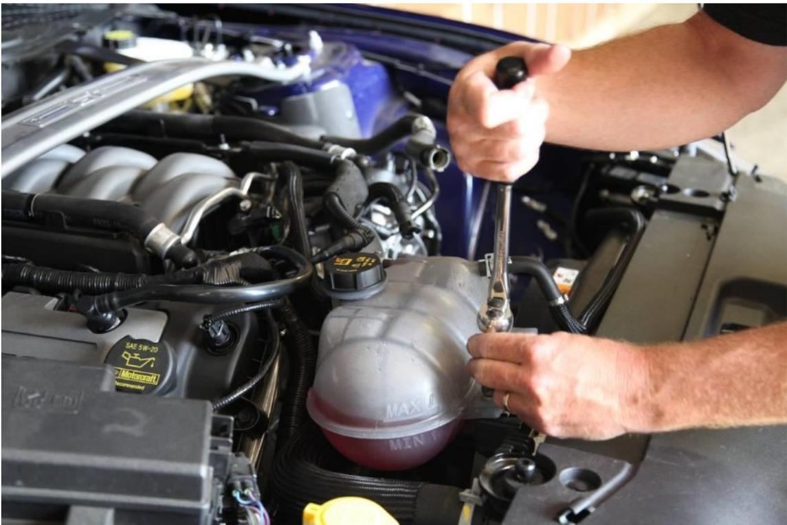
14 Install coolant reservoirs onto relocation bracket using factory bolts.
