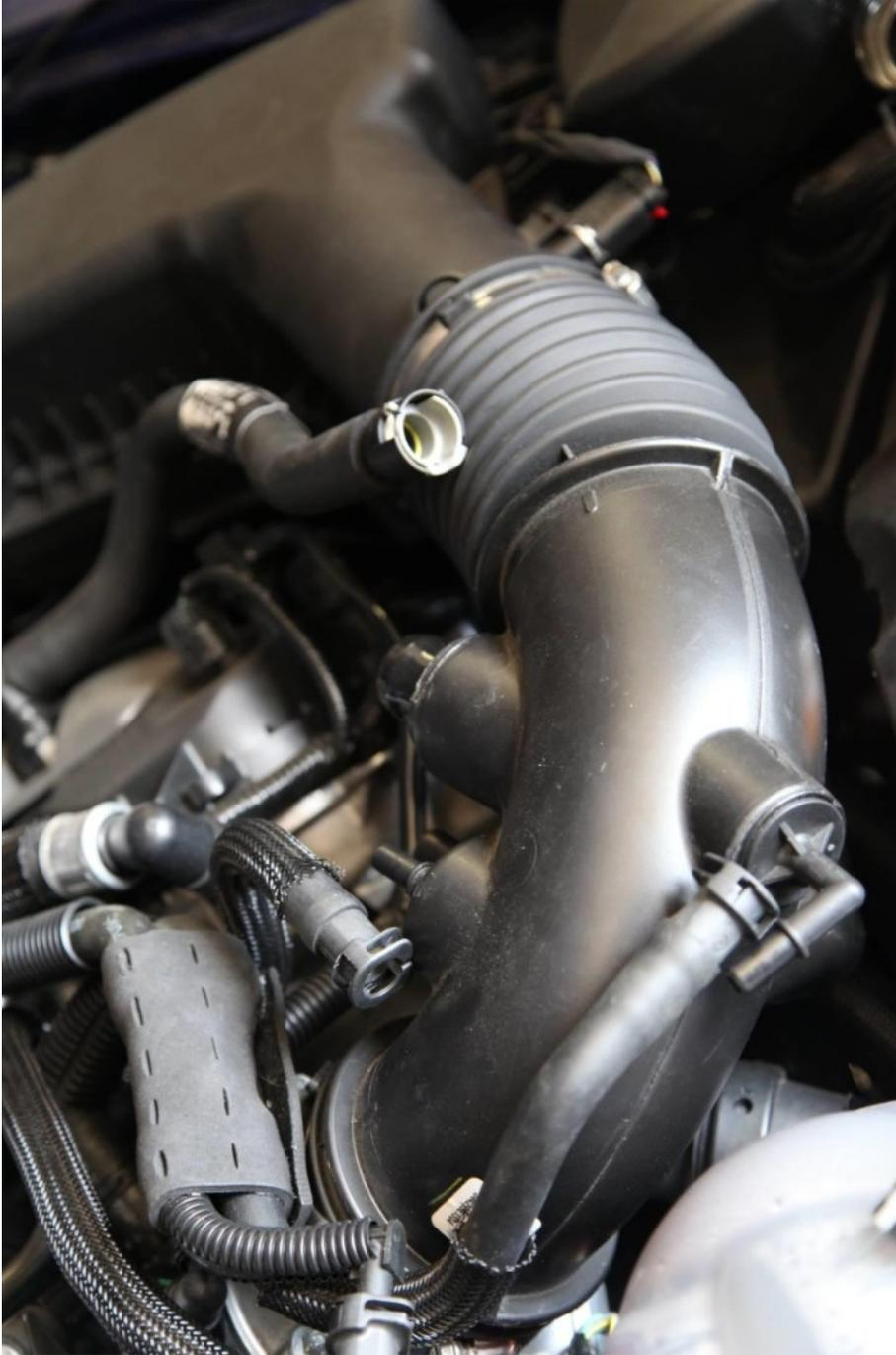
11: Remove sound tube from intake tube.
