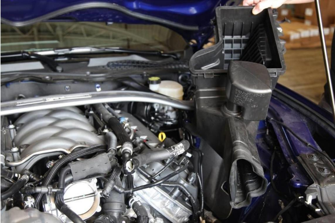
7: Remove intake tube clamp at throttle body
