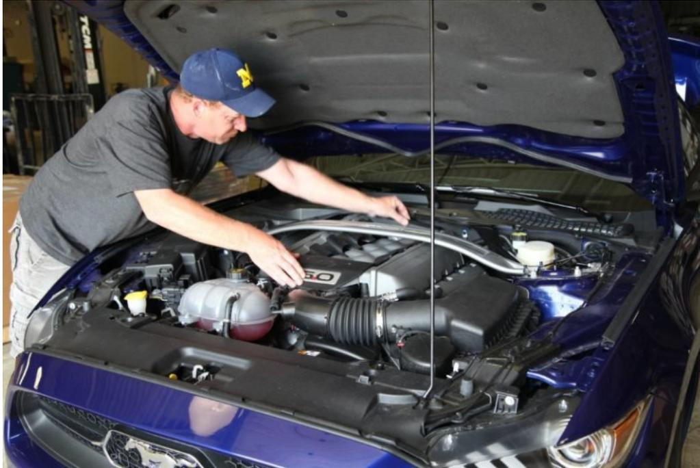
2: Disconnect Mass airflow sensor connector
