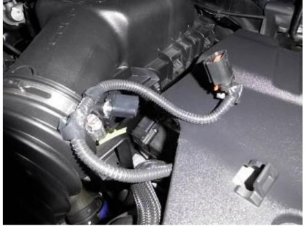
3: Remove hose clamp at air box next to mass airflow sensor
