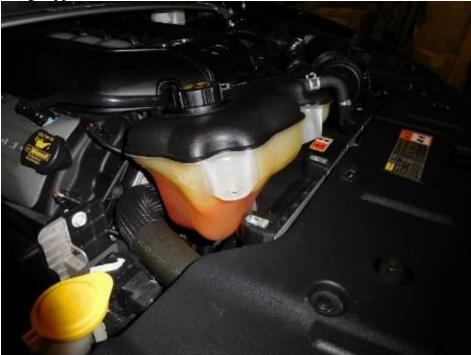
14 Install coolant reservoir onto relocation bracket using factory bolts.
