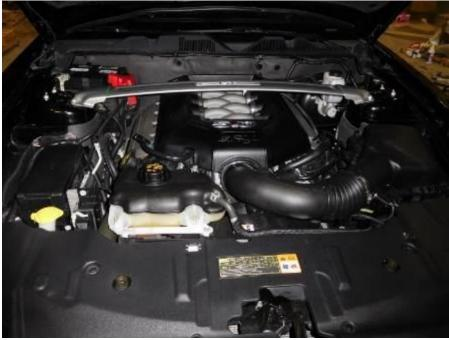
Step1: Remove strut tower brace and decorative engine cover.
