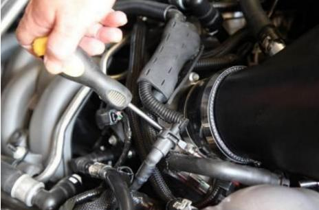
20: Make sure MAF is correctly oriented and placed, then tighten down two 5" hose clamps.
