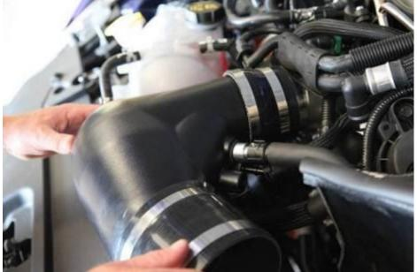
19: This step in very important. Make sure that throttle body coupling is pressed firmly and completely onto throttle body. If done correctly the large intake elbow will be touching the top of the fan shroud, this will ensure proper hood clearance. Tighten throttle body clamp.
