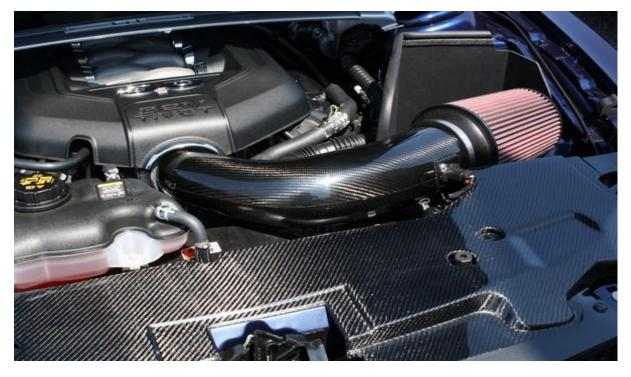
Oil Filter: The frequency you should clean your filter will depend on your driving conditions. It is recommended to check your filter at every oil change or 3,000 miles. If there is a build up of dirt as thick as the wire mesh, then it's time to clean your filter. As dirt builds up on your filter, the restriction of the airflow also increases. More frequent cleanings will improve your fuel economy and your vehicle's performance.
