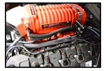
142. Install the supplied 3/8" ID hose from the brake booster to the lower quick connect fitting on the supercharger inlet. Push until it clicks into place.
