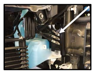
183. (Complete kits only) Whipple complete kits connect to the IMRC wires to turn on the IC pump and fan when applicable. Competition kits use a common fuse in the fuse panel, therefore the harness is different. Connect the supplied 2-way connector of the intercooler/fan control harness to the 2-way passenger side IMRC connector (yellow/grey and green wires). Route to the fuse box area for later installation.
