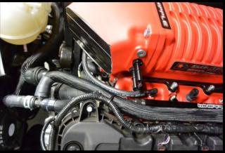
138. Install the supplied coolant vent line with dual 90deg's. Use the factory pinch clamps to secure hose in place.
