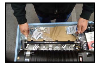
86. Install the supplied (8) manifold orings into the Whipple intake manifold.
