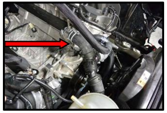
75. Install the factory coolant overflow hose to the new supplied tee fitting on the driver side. Secure using factory pinch clamp.
