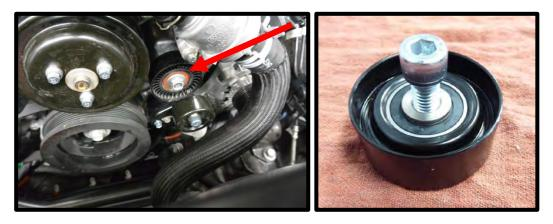
111. Install the supplied (1) 10mm x 25mm SHCS through the idler plate and supercharger front support. Install hand tight. Torque the 10mm bolt to 25 lbs-ft. and the (5) 8mm idler plate bolts to 18 lbs-ft.
