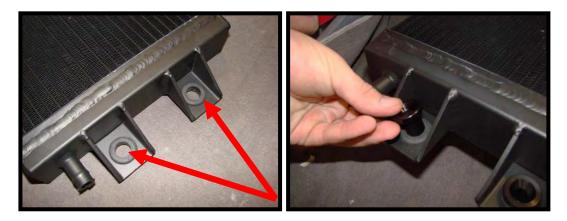
130. Install the LTR brackets to the LTR using the supplied (4) 8mm x 35mm FHSCS bolts through the aluminum heat exchanger spuds (5mm allen socket).
