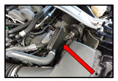
37. Carefully disconnect the factory fuel feed hose from the fuel rail. The fuel system may still have pressure, use protective eyewear and multiple rags to catch any possible fuel leak. To release, press the blue safety latch and pull the fuel fitting away from fuel rail.
