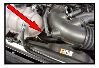
16. Remove the pinch clamp securing the sound resonator tube to the inlet tubing. Remove rubber line from inlet tube.
