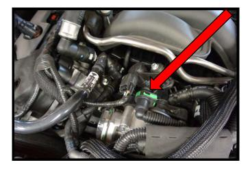
29. Remove the EVAP tubing from driver side valve cover (remove support from valve cover) and down below brake booster.
