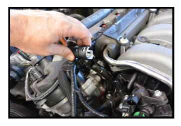
34. Remove the quick connect fitting on the heater tube, drivers side. Push hose to the back of the engine for later use.
