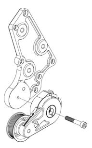
115. Install the supplied (3) smooth idler pulleys #36101 to the idler plate using the (3) step spacers. Sandwich the idler pulley to the step spacer using the supplied (3) step washer and (3) ½"-13 x 1 ¾" SHCS and torque to 30 lbs-ft. using a 3/8" allen socket. Use light amount of anit-seize on threads.
