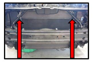
124. **(Dual fan installation)** Install the supplied (4) rubber strips to the bottom flat portion of the fan mount brackets. Clean the brackets with soap and water. Remove the protective tape from the rubber strip and install to the bracket.
