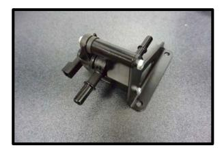
97. Install the supplied 6AN viton oring (#906) to 9.89mm to supplied 6AN quick connect fitting. Install this fitting to the EVAP solenoid billet adapter.
