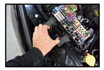
179. Using the supplied plastic push pin, sandwich the relay and fuse holder to the passenger side inner fender hole. Push pin in to lock in place.
