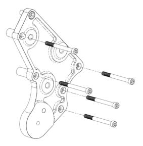
108. Install the supplied adjustable idler assembly to the factory spring loaded tensioner position. One side has a dowel pin which locates the base. Install the adjustable arm to the stock location using the stock spring loaded tensioner bolt. Torque the factory bolt to 18 ft-lb.
