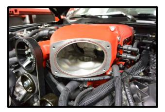
172. **(Stock throttle body)** Install throttle body adapter to supercharger inlet using the supplied (4) 6mm x 14mm FHCS (4mm allen socket). Torque to 88 lbs-in.
