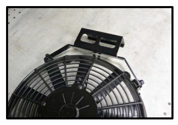
126. (**Dual fan installation**) Carefully set both fan assemblies on top front of the LTR, space these evenly before installing.
