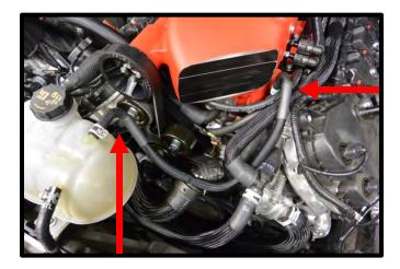
139. Install the (2) supplied 6AN viton oring (#906) to the (2) 6AN to 3/8" quick connect fittings. Install these fittings to the passenger side lower 6AN fittings on the inlet using an 11/16" socket.
