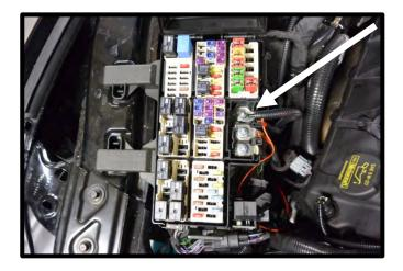
182. Remove the ground bolt from the passenger, radiator core support using an 8mm socket. Install IC pump relay ground eyelet here. Secure with factory bolt using an 8mm socket.
