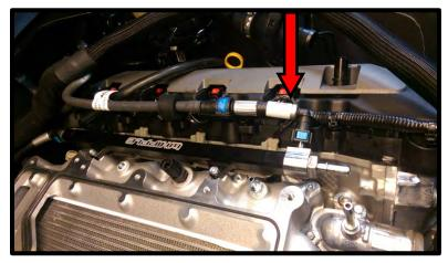
95. Install the factory EVAP solenoid to the supplied billet adapter. Mount to the adapter using the supplied (2) 6mm x 25mm SHCS and torque to 106 lbs-in using a 5mm allen socket.
