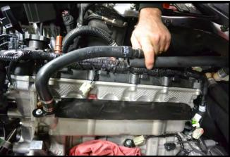
63. Using a pair of wire cutters, cut the safety clamp off the passenger side heater hose (to remove restrictor).
