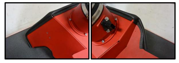
162. Install the airbox into the vehicle, leave loose for now.
