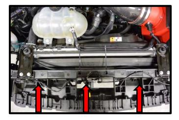
186. (**Dual Fan installation**) Connect the 12V eyelet to the 3<sup>rd</sup> power stud (same as IC pump previously installed). Connect the orange turn-on wire to the IC pump harness orange wire. Use the supplied steel bracket to use previously installed push pin to secure relay and fuse. Connect the ground wires as stated below. Route the wires down on the passenger side of radiator. Connect dual fan 2-way's to fan relay harness 2-way's. Zip tie wires for clean installation.
