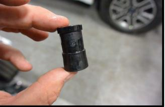
64. Install the restrictor into the supplied 90deg rubber hose. Install hose over the heater tube you just installed to push restrictor to proper height. Once there, remove hose from heater tube and install the supplied safety clamp. Use a pinch tool to secure safety clamp on restrictor.
