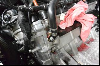
67. Remove the factory sheaving off the passenger side heater hose. Using the supplied hose and barb fitting, cut factory hose length so the hose will go straight back towards firewall. Once cut to proper length, slide the supplied sheaving on the supplied 90deg hose and (2) pieces of rubber heat shrink (for later install). Install the supplied shrink clamp over factory heater hose. Install the factory heater hose to the coupler. Use a heat gun to secure the shrink clamp.
