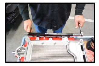
84. On the driver side front fuel rail inlet, install the supplied stainless steel banjo fitting hand tight. Apply light amount of grease to banjo fitting oring for ease of installation.
