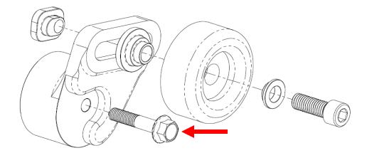
109. Install the supplied idler pulley to the adjustable idler position using the supplied step spacer against the adjustable idler arm. Sandwich the smooth idler pulley (#36101) to step spacer and the supplied step washer to front side of idler. Install the supplied "tee" nut to the back side with the offset hole facing the driver side. Secure with the supplied ½"-13 x 1 ¾" SHCS and torque to 30 lbs-ft. Use light amount of anit-seize on threads.
