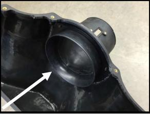
157. (Complete Kits) Install the supplied snorkel to the airbox lower half. Use the supplied (4) flanged BHCS to secure.
