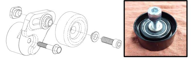
110. Remove the factory plastic smooth idler pulley from the engine. Replace with the supplied steel idler pulley. Use the factory fastener to secure. Torque to 17 lbs-ft.
