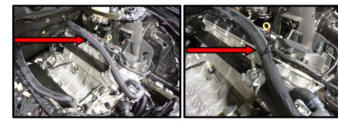
73. Reinstall the thermostat housing junction quick connect fitting to the thermostat housing junction until it locks in place.
