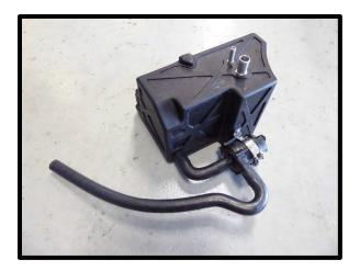
152. Mount the intercooler reservoir to the driver side below headlight. Secure using the (2) holes coming from the fender and one (1) from radiator support bracket. Secure the upper using the supplied (2) 8mm x 20mm hex head flange bolts with the flat washer against the head using a 13mm socket. Use the supplied (1) 8mm x 16mm SHCS and (1) 8mm AN washer from the bottom side of radiator support bracket.
