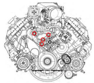
105. Install the (5) support stands to the front idler plate. These are loose fit, therefore you must tilt backwards during installation or the stands will fall. You can use masking tape to help hold in place during installation if installation becomes difficult. Each support stand is marked with an identifying number, as well as the idler plate for ease of placement. Assemble together with the number facing out for future reference.
