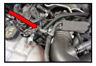
20. Remove the vent line coming from the driver side IMRC vacuum line by squeezing the connector and pulling away from hose.
