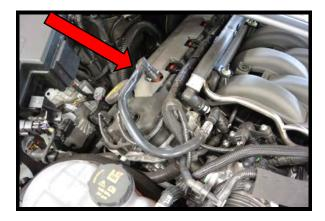
19. Remove the passenger side IMRC vacuum line coming from the intake manifold by squeezing the connector and pulling away from brake booster hose.
