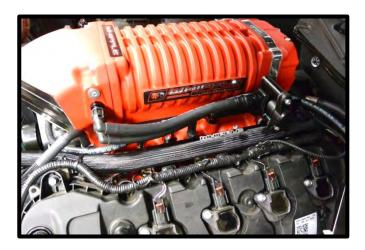
144. Install the (1) supplied 6AN viton oring (#906) to the (1) 6AN to 5/8" quick connect fittings. Install this fitting to the driver side 6AN fittings on the inlet using a 7/8" wrench.
