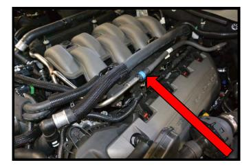
38. Remove the (4) bolts from the top of the intake manifold that secures the (2) heater hose trays. Use a 10mm deep well socket. Once bolts are removed, remove tray and foam material.
