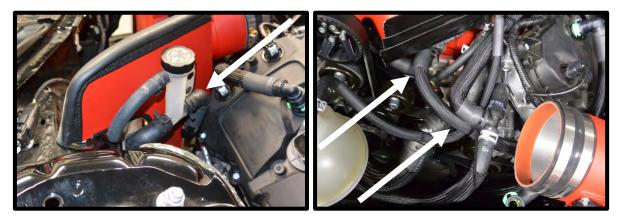
169. Install the supplied 3/8" ID IC vent line (COYO-1500) and the ¾" ID IC rubber hose (COYO-1400) to the filler neck. Secure both with supplied pinch clamps. Route both below the airbox, to the IC reservoir. Secure both ends with supplied pinch clamps. Use multiple zip-ties to secure hoses together. **Watch for hose kinks!**
