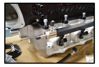
85. On the driver side rear fuel rail outlet, install the supplied stainless quick connect fitting with oring hand tight. Apply light amount of grease to oring for ease of installation. Using a 7/8" wrench on the banjo fitting and a ¾" wrench (or deep socket) on the outlet fitting, tighten both. Make sure to not torque the injectors over while tightening the fittings.
