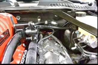
143. Install the supplied 3/8" ID x 21 hose from the factory EVAP barb fitting located on the driver side lower inner fender (below brake booster) and route to the EVAP quick connect fitting. Push until it clicks and locks into place.
