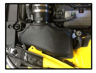
178. Lift the fuse box so it's slightly up by squeezing the (2) pins on the fuse box lid.
