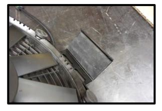
125. (**Dual fan installation**) Install the (4) brackets to the fans by sliding the square tab into the fan notch and the steel channel bracket will slide on the outside. The angled side will face the fan. This slides together easier if the bracket is facing slightly up. Once these are lined up, push until the seat together. Repeat on the other (3) brackets. Leave nyloc nuts loose for now.
