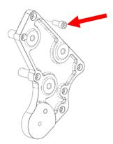
112. Torque the (10) 6mm SHCS manifold bolts in the following pattern using a 5mm ball head allen socket. First pass: 88 lbs-in. Second pass: 106 lb-in.
