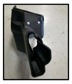
158. (**Competition Kits**) Using the supplied MAF housing and 123mm plastic venturi ring, mount to the new cold air box with the (4) 6mm x 16mm SHCS (5mm allen ball socket). Torque to 75 lbs-in.
