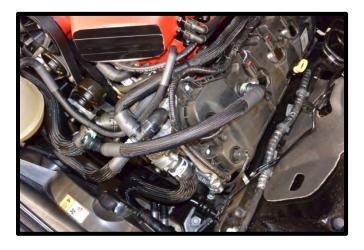
147. Install the supplied ¾" ID molded hose (#COYO-1300) from the IC top fitting (outlet) to the airbox area for later installation. Secure end with supplied pinch clamp. Secure this line to the "Tee" branch from the engine coolant lines using a zip-tie. Make sure to give 1" of clearance from the smooth idler pulley.
