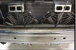
135. With the LTR mounted, mark the centerline of the LTR fitting and horizontally center of the plastic radiator (passenger side) shrouding. Using a 1 ½" hole saw, drill a hole through the plastic shrouding. Install the supplied 1 ½" rubber grommet into this hole.
