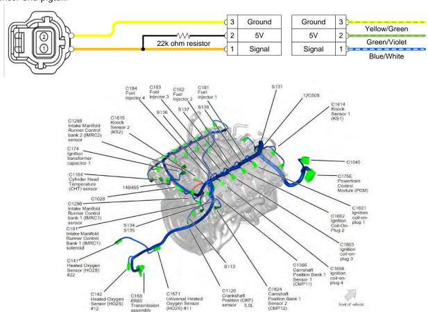
78. (Complete kits) Connect the supplied 2-way connector of the intercooler/fan control harness to the 2-way passenger side IMRC connector (yellow/gray and green wires). Route to the fuse box area for later installation.
