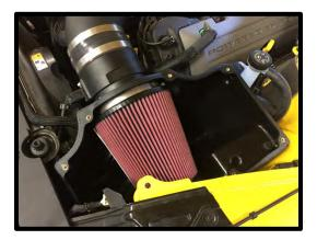
165. (**Competition Kits**) Install the (2) 1 ½" aluminum filler neck stands to the airbox using the supplied (2) 6mm x 12mm flanged BHCS (4mm allen socket).
