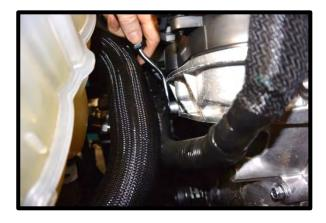
56. Using a 10mm socket, loosen each knock sensor and rotate outwards until connector almost touches block. Once rotated, torque to 18 lbs-ft. **NOTE:** Should be .100" away from touching block/head.
