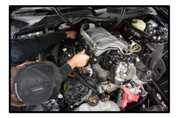
48. Clean the intake manifold to cylinder head surface using carb cleaner or acetone. Install tape over the exposed ports until manifold installation.
