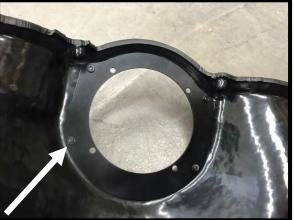
156. (**Complete Kits**) Using the supplied MAF housing and 123mm plastic venturi ring, mount to the new cold air box with the (4) 6mm x 16mm SHCS (5mm allen ball socket). Torque to 75 lbs-in.
