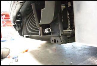
154. Once plastic shrouding is notched, use the supplied pinch clamps to secure the 3/4" ID x 20" hose from IC pump outlet to LTR inlet. The image shows the hose, it must sit in the channel just behind the air dam (below fog light). Make sure to not allow any kinks.
