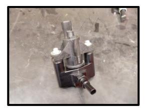
96. Install the EVAP solenoid assembly to the formed steel bracket using the (2) 6mm x 15mm SHCS torque to 106 lbs-in using a 5mm allen socket.
