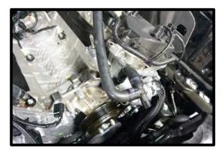
71. Using the supplied hose coming from the supplied tee fitting, route between cylinder head and water neck. Cut factory hose length so the hose will go straight back towards firewall. Once cut to proper length, slide the supplied sheaving on the supplied hose and (2) pieces of rubber heat shrink (for later install). Secure with supplied pinch clamp.
