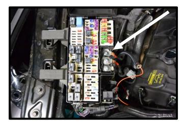
181. Install the IC pump relay power eyelet (red wire) to the power stud you just removed the nut. Use a 10mm socket to secure stock and IC power wire. Torque to 88 in-lbs.
