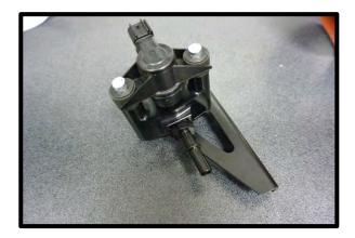
98. Install the (2) supplied manifold orings into the oring groove. Use silicone/grease in receiver groove to help oring stay in place.
