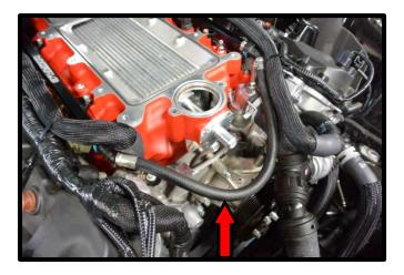
94. Install the supplied male to female fuel line to the factory supply line coming up on the driver side of engine by pressing until they click and lock into place. Connect the male end to the factory line and the 90deg female end to the banjo fitting.
