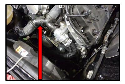
42. Remove the thermostat housing hose using a pinch clamp tool. Pull away from thermostat housing.
