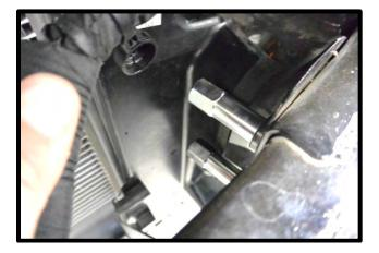
132. (Stage 2 heat exchanger installation) Remove the factory plastic support clamps from the wire harness. Use a flat blade screw driver to open. Use a plastic pin pry tool to remove the clamps from the vehicle.
