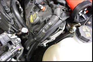
137. Install the supplied ¼" ID bypass actuator to the bypass nipple and ¼" nipple above first cylinder on driver side.
