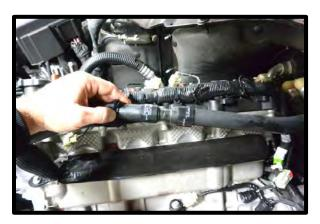
68. Slide the supplied sheaving over the passenger side heater hose along with the rubber heat shrink. Use the heat shrink to secure sheaving on both sides of hose. It's a good idea to run the heat gun over the sheaving material to secure it tighter to the hose then follow with shrinking the heat shrink to cover the ends of the sheaving for a professional looking installation.
