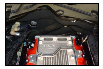
93. Install the supplied fuel cross over line (1 of 2) to the front fuel fittings by pressing until they click and lock in place.
