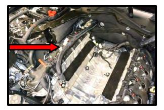
69. Install the supplied driver side heater tube to driver side of block (bracket has step in it). Install the supplied oring to the tube and apply light amount of grease to oring surface. Install tube into block and secure with the factory bolt using an 8mm socket. Torque to 89 lbs-in.
