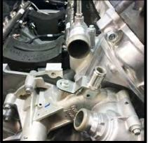
70. Install the supplied tee assembly to the driver side heater tube you just installed. Secure with the supplied pinch clamp. **NOTE:** Short end of 90deg goes on heater tube, long end goes on tee fitting.
