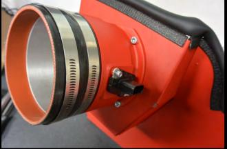
159. Install the factory MAF sensor element into the new MAF housing using the supplied (2) 4mm x 6mm SHCS. Torque to 17 lbs-in. \*\***DO NOT USE STOCK BOLTS\*\***.
