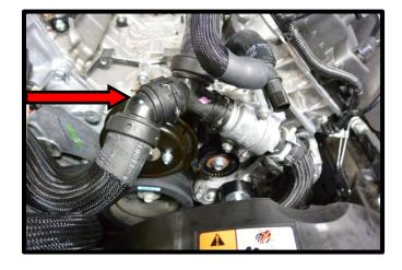
74. Reinstall the water neck to thermostat housing junction hose to the water neck. Secure by releasing the factory pinch clamp.
