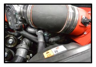
176. (Whipple 132mm Crusher throttle body) Install the supplied 5" ID x 2" silicone hose over air inlet tube so it's not hanging over the end. Install the air inlet tube between the MAF and throttle body. Slide silicone hose over throttle body. Secure all ends with the supplied #80 hose clamps. \*\*Never over torque the clamp to secure the silicone hose to the MAF housing, this can distort the MAF and lead to running issues. 45-55 lbs-in is recommended.
