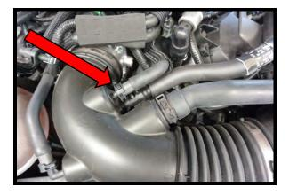
21. Disconnect the factory MAF connector by pulling back on the safety lock, then squeezing the unlocking tab and pulling back.
