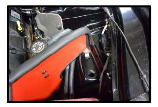
164. (**Complete Kits**) Install the supplied high-flow air filter and clamp over the 123mm venturi ring. Once in place, secure hose clamp using a 5/16" nut driver. You may need to lift the box to get the filter in. Once filter is in place, install the supplied (1) 6mm x 15mm SHCS and 6mm washer to secure airbox to inner fender. You will have to rock the airbox and lift to get filter in place.
