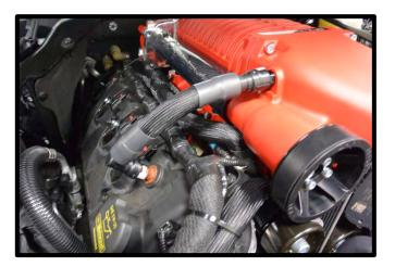
146. Install the supplied 5/8" ID x 15" hose to the driver side valve cover. Push until it clicks and locks into place. The other end will be installed in inlet tube later.
