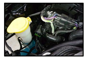
180. Remove the 3<sup>rd</sup> (from front) nut from the power stud using a 10mm socket.
