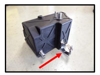
151. Install the intercooler pump to the water reservoir using the supplied clamp (leave slightly loose to position after hose installation). Install the supplied 90deg rubber hose and pinch clamps to reservoir and intercooler pump. Once pump is in position, tighten clamp holding IC pump to reservoir. Note: Make sure pump outlet is facing directly out (not up or down).
