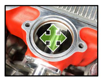
102. The supercharger must be filled with oil prior to use. This supercharger is shipped without oil inside. The oil is in a separate bottle supplied with your kit and is pre-measured for the exact amount of oil.
