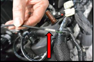
121. Install the supplied ground wire with eyelet using the 8mm x 25mm hex head flanged bolt to secure. Torque to 15 lbs-ft
