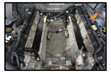
49. Remove the driver and passenger side heater tubes from engine by removing the (1 bolt per) bolt using an 8mm socket.
