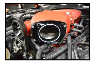
173. (Whipple 132mm Crusher throttle body) Install throttle body to supercharger inlet using the supplied (3) 6mm x 25mm SHCS and (1) 6mm x 50mm SHCS using a 5mm allen socket. Torque to 88 lbs-in.
