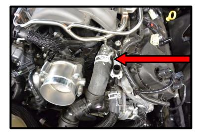
41. Remove the quick connect water fitting from the water neck to thermostat housing tee. Pull the locking metal wire, then pull connector back away from tee.
