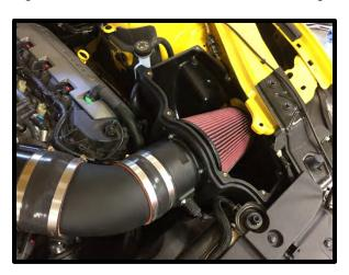
177. (Complete Kits) Install the supplied airbox lid using the supplied (7) 6mm x 10mm flanged BHCS.
