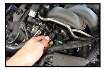
28. Remove the EVAP vent line quick connector from the EVAP solenoid by pushing the (2) locking tabs away and squeezing the tab, then pull away. Pull this line away from engine (goes down to driver side lower firewall area).
