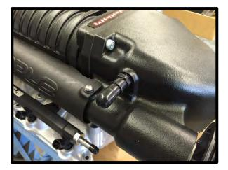
145. Install the supplied 5/8" ID x 6.5" hose to the passenger side valve cover. Connect other end to the supercharger inlet quick connect fitting. Push until it clicks and locks into place.
