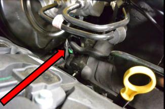
30. Remove the manifold vent hose next to the EVAP, use a pinch clamp tool to remove pinch clamp and hose.
