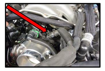
31. Remove the vent hose coming from the thermostat housing fitting by removing pinch clamp. Remove vent line from overflow tank by removing pinch clamp using a pinch clamp tool.
