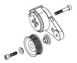
114. Install the spring loaded tensioner to idler plate, locating the tang into position. Secure with the supplied 10mm x 60mm SHCS. Use light amount of anit-seize on threads. Torque to 25 lbs-ft.
