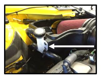
168. Connect the ¾" ID molded rubber hose you previously installed to the IC top (outlet) fitting and connect to the IC filler neck. Secure with supplied pinch clamp.
