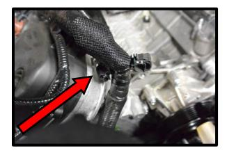
55. Using a plastic pin pry tool, remove the wire harness support from the passenger side of engine block.
