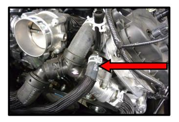
40. Remove the water neck hose using a pinch clamp tool. Pull away from water neck.
