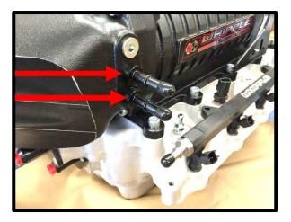
140. Install the (1) supplied 6AN viton oring (#906) to the (1) 6AN plug. Install the fitting to the passenger side upper hole on the inlet using an 11/16" socket.
