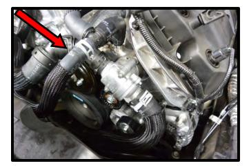
76. **(Competition kits cover all)** Cover the remaining (1) IMRC solenoid and (1) IMRC position sensor connectors with electric tape and secure to the factory loom at the back of the engine.
