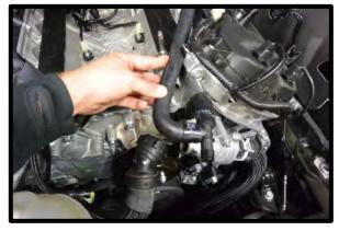
72. Slide the supplied sheaving over the driver side heater hose along with the rubber heat shrink. Use the heat shrink to secure sheaving on both sides of hose. It's a good idea to run lightly run the heat gun over the sheaving material to secure it tighter to the hose then follow with shrinking the heat shrink to cover the ends of the sheaving for a professional looking installation. Secure hose to wire harness with zip-tie for easier installation. More zip-ties will be installed later.
