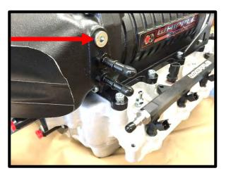
141. Install the supplied 3/8" ID hose from the EVAP to the top quick connect fitting. Push until it clicks and locks into place.
