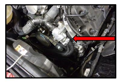
43. Remove the (2) bolts securing the thermostat housing body together using a 8mm socket.
