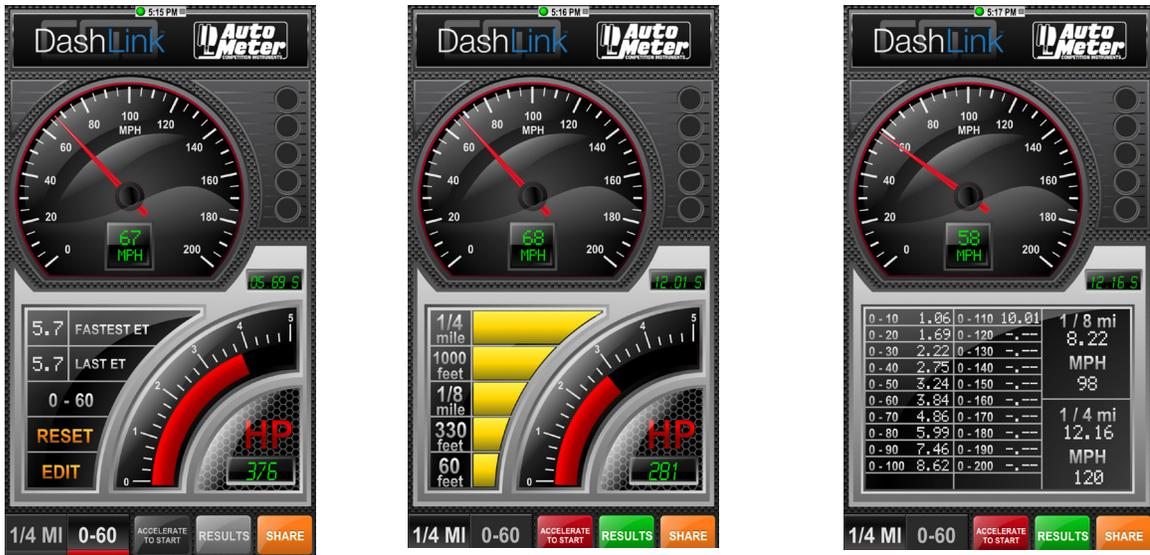
The 0-60 timer will track 0-60 time by default. When the vehicle starts moving, the timer starts. It will show the time when the vehicle reaches 60. The edit button can be used to change it to any start speed and stop speed (EX: 30-50 MPH). The time will start when the vehicle reaches the starting speed and will stop at the stop speed. To try again, slow down below the minimum speed and start again. The reset button will clear the Fastest and Last ET numbers.
