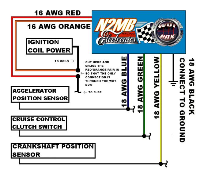
Figure II: Installation Diagram
