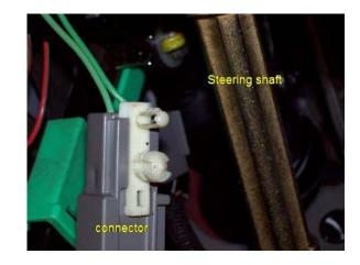
11) Route the GREEN WOT Box wire to this location, using zip-ties to secure along the way, and splice the GREEN WOT Box Wire into the PIN#1 (BOTTOM PIN, TOWARDS REAR OF VEHICLE) LIGHT GREEN wire, making sure that the original connectivity of the wire is maintained.
