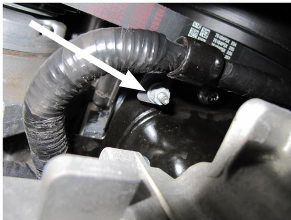
Fig. 11-a: Wiring Harness Mounting Location (pass. side shown, driver side similar)
