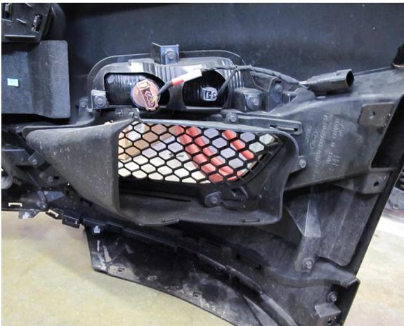
Fig. 12-m: Remove Transmission Cooler Duct
