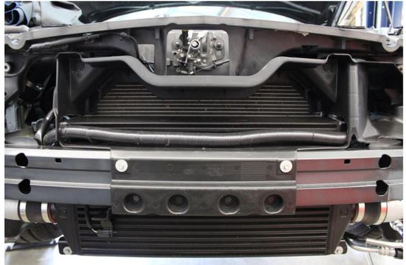
Fig. 5-e: Modified Radiator Shroud
