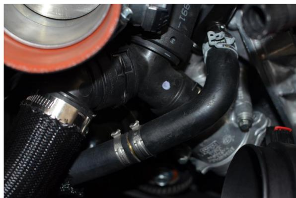
Fig. 7-n: 3/4" 90° Hose Elbow
