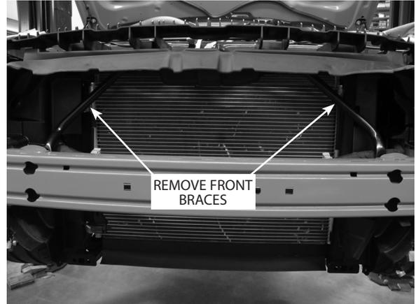
Fig. 5-a: Remove Front Braces
