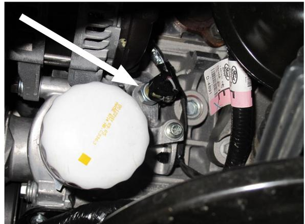
Fig. 10-e: OEM Oil Pressure Sensor
