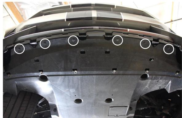
Fig. 1-g: Remove Front Belly Pan Screws
