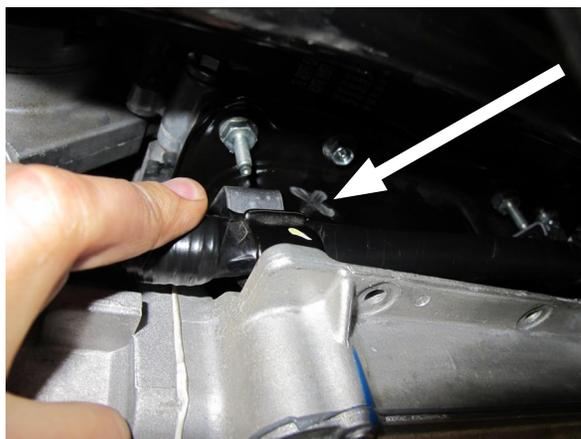
Fig. 11-b: Oil Drain Fitting Installation Location
