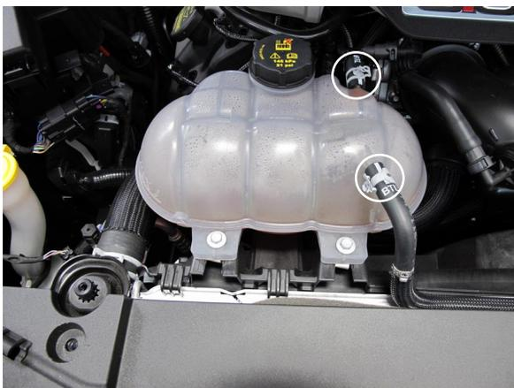
Fig. 1-p: Coolant Reservoir
