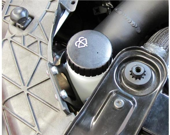
Fig. 12-g: Mount Remote Fill Bracket
