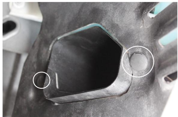
*Fig. 1-c: Remove Fender Liner Fasteners*
