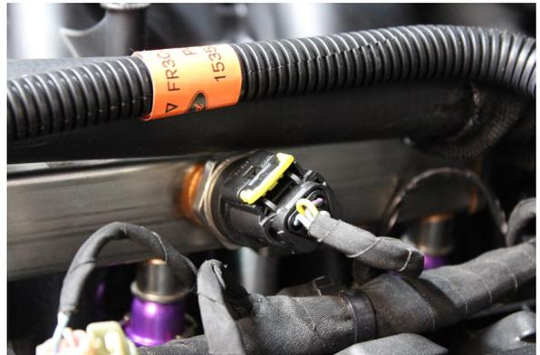
Fig. 6-h: Aluminum Fuel Rail Spacers
