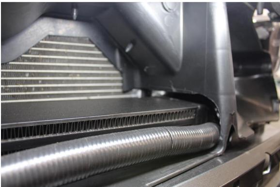
Fig. 5-d: Modified Upper Shroud Section
