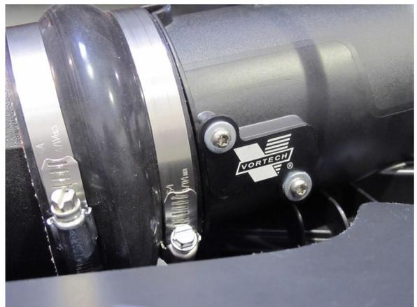
Fig. 8-c: Air Inlet to Airbox Connection; MAF Port Cover
