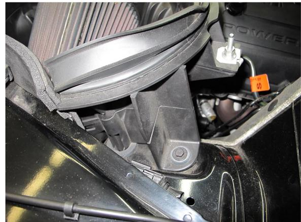
Fig. 1-n: Unplug MAF & Remove Air Inlet Assembly
