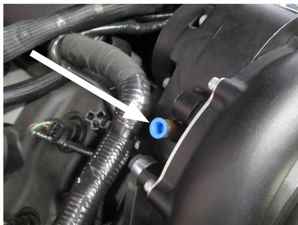
Fig. 10-a: Supercharger Oil Feed Location
