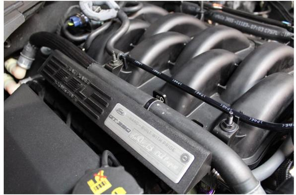
Fig. 6-b: Hose Guide Removal
