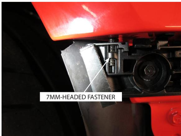
Fig. 1-h: Bumper Corner Fastener
