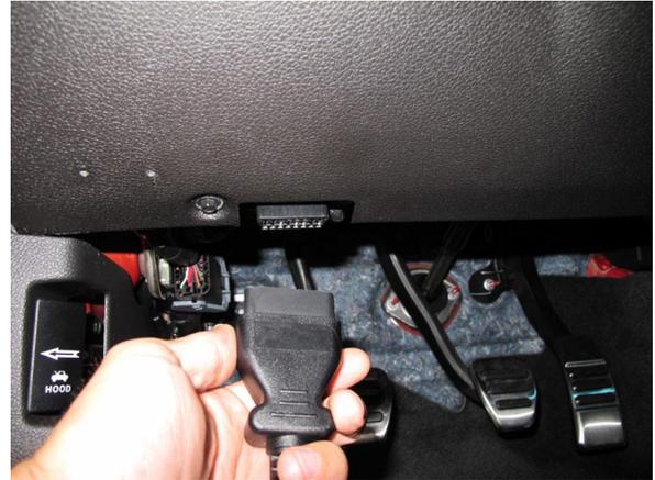
Fig. 12B: OBD2 Connector and Port
