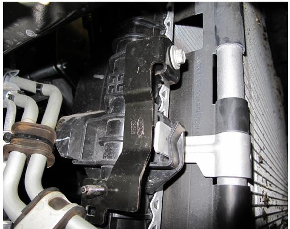
*Fig. 12-c: Remove Transmission Cooler Lines Mount From Radiator*
