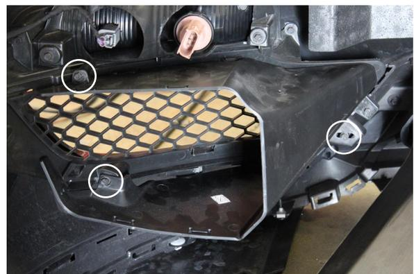
Fig. 5-o: Remove Oil Cooler Duct
