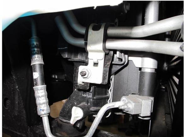
*Fig. 12-b: Remove Transmission Cooler Lines From Mount*
