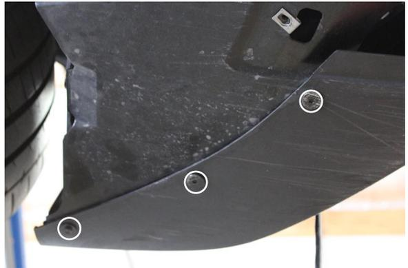
Fig. 1-f: Remove Screws Securing Front Bumper Corners
