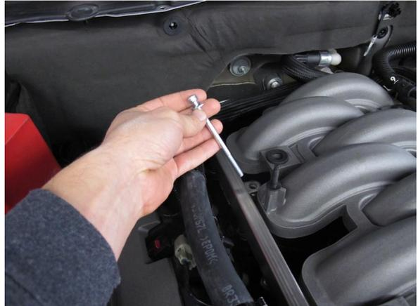
*Fig. 6-m: Re-securing Fuel Rails*
