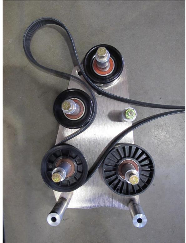
*Fig. 3-c: Belt Routing
