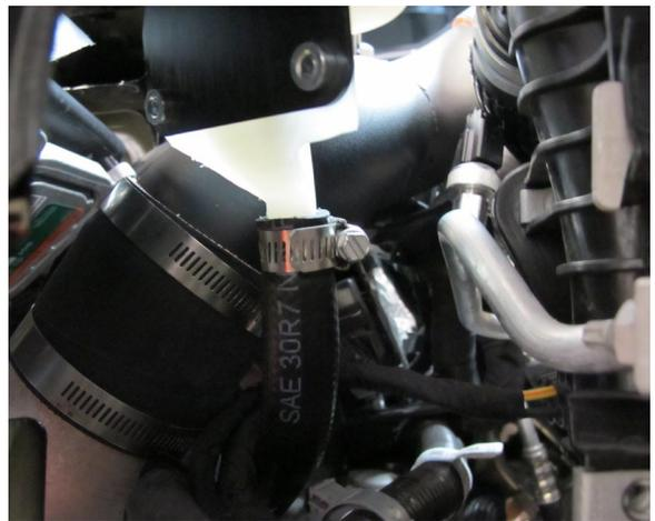
Fig. 12-k: Secure 5/8 Hose To Remote Fill Reservoir
