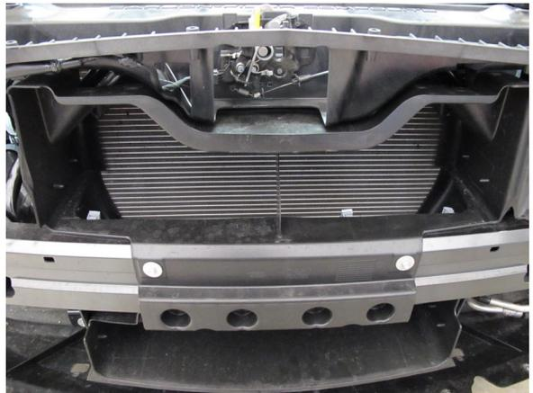
*Fig. 1-j: Remove Radiator Shroud*
