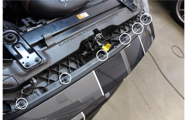
*Fig. 1-a: Remove Bumper Cover Fasteners*
