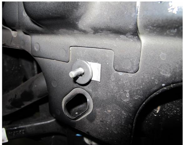
Fig. 12-i: Install 5/16 Washer To Mounting Stud
