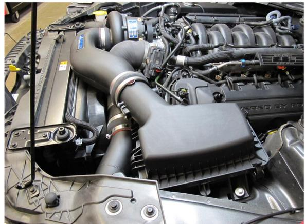
Fig. 8-e: Connect Inlet Duct To Air Box
