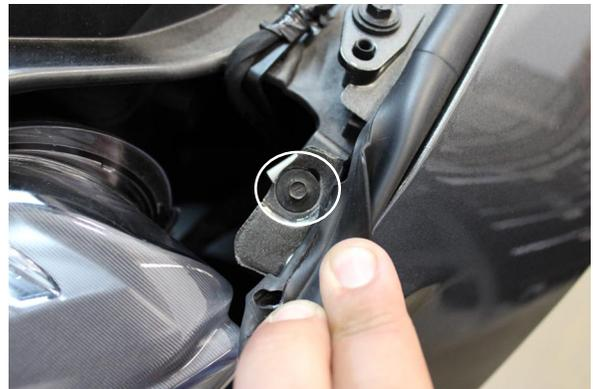
*Fig. 1-b: Remove 5.5mm-Headed Fastener*
