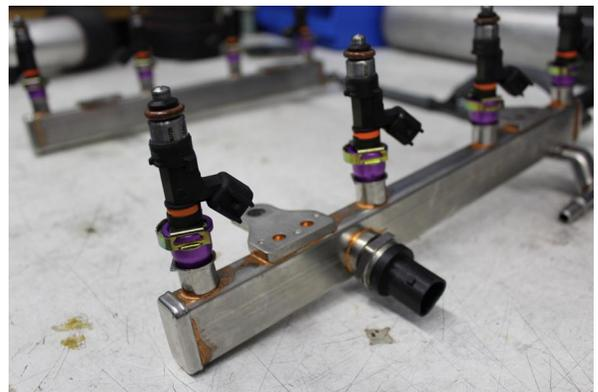
Fig. 6-k: Fuel Rail / Injector Assembly Detail
