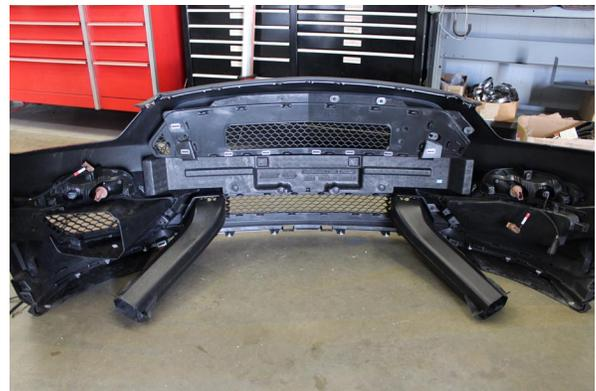
Fig. 5-n: Remove Brake Cooling Ducts
