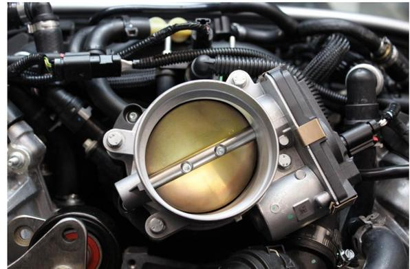
Fig. 3-n: Mounted Throttle Body
