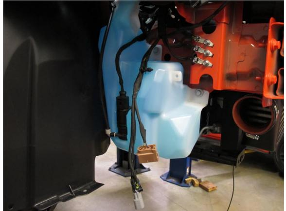
*Fig. 12-a: Remove Windshield Washer Reservoir*
