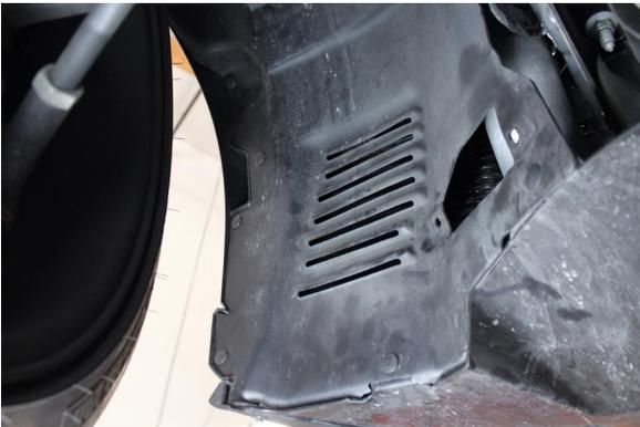
*Fig. 1-d: Remove Fender Liner Fasteners*
