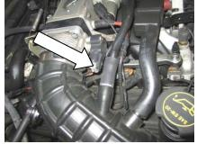
9. Reattach the factory air duct and breather hoses. Use the 5/8 breather hose to connect the factory hard line to the fitting installed in step #8.
