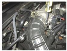
1. Disconnect the negative battery cable and loosen the clamps holding the factory duct in place.
