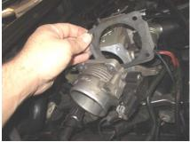
5. Remove the factory throttle body gasket.
