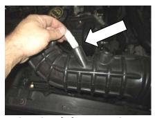
8. Place the 5/8 fitting into the factory air duct nearest the throttle body.
