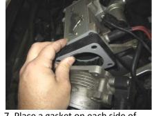
7. Place a gasket on each side of the spacer and install with the curved edge of the fins facing the throttle body.
