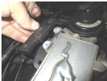
10. Install the cable extension bracket into the factory location using the supplied allen screws.
