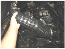
3. Remove the factory air duct.
