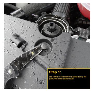
Use a knife or screwdriver to gently pull up push pins in the radiator cover
