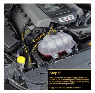
Now you can see the installed system and just double check all the fittings and connections are final tightened and don't forget to clean up when you are completed your install.
