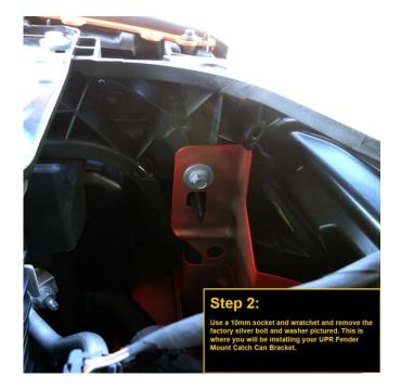
Use a 10mm socket and ratchet to remove the factory silver bolt and washer pictured. This is where you will be installing your UPR fender mount catch can bracket.
