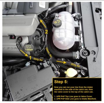
Now you can run your line from the intake manifold to the side of the catch can, then the valve cover to the top of the catch can.
