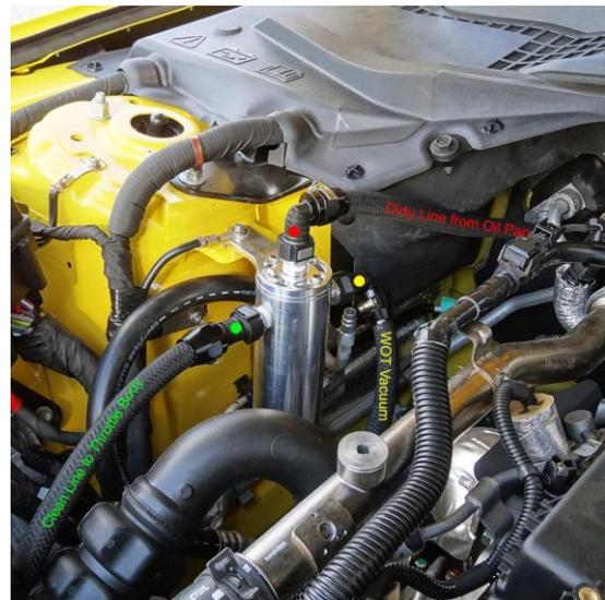
Mount the catch can to the passenger side strut tower under the ground strap bolt as shown. Remove the OEM line from the throttle body to the oil pan. Heat the ends of the line to remove the OEM connectors.
