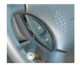
2. Make sure to leave the rubber switch covers in place when installing the new cruise control buttons.
