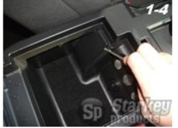
Remove e-brake access cover with a flat head screwdriver.
