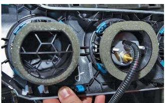
4. Before reinstalling the instrument cluster bezel, run all necessary wiring and hoses based on the gauge selection. A hole will need to be drilled in the duct work, in order to feed the wires into the back of the vent pod. The picture shown illustrates the hole for a vacuum hose and the necessary wiring.
