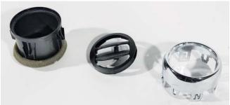
4. Once the trim ring has been removed, carefully cut out the honeycomb center section off of the rear of the vent. Using a suitable cutting tool, clean any burrs or high spots. The amount of material removed will depend on the gauge (not included) that is being installed in the vent body.
