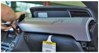
2. Locate the four (4) locking tabs which retain the inner vent assembly to the cluster bezel. Select the vent to be replaced with the vent pod for the gauge location, and carefully depress all four (4) tabs to release the inner vent assembly.
