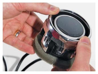
Locate and align the inner vent housing assembly with the cluster bezel. Reinstall the inner vent housing until each of the four (4) locking tabs have locked into position. The trim ring should be seated flush with the cluster bezel and locked securely into position.
