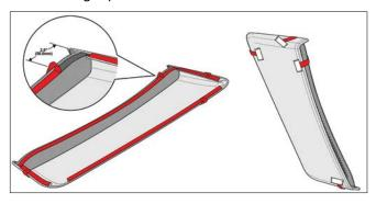
Install the side scoop onto the body side using the directions on the template. Do not allow the exposed double-sided tape to adhere to the sheet metal until the side scoop is properly aligned, then press down.
