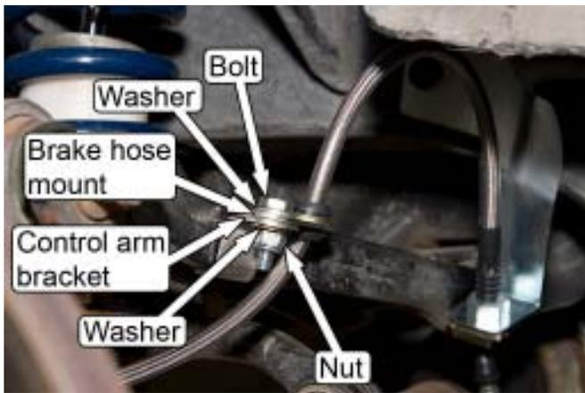
13. Remove the rubber brake hose plug from the OEM brake hard line and connect it to the end of the MM Stainless Steel Brake Hose retained in the MM Frame Rail Bracket, using a 12mm flare nut wrench, then tighten the fitting.
