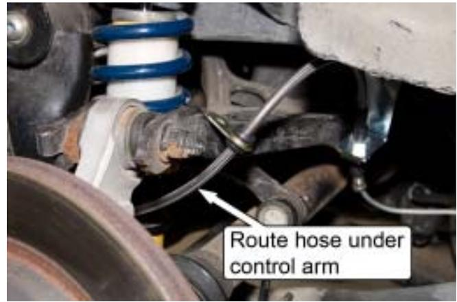
8. Attach one of the supplied MM Stainless Steel Brake Hoses to the MM Frame Rail Bracket. The hose end fitting with the groove must pass through the top side of the hole on the lower end of the MM Frame Rail Bracket.
