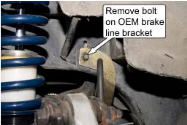
5. For 2003-2004 Mustang Cobra, unbolt and remove the rear upper control arm brake hose bracket from the control arm. Use a flat-blade screw driver or pliers to help spread the bracket legs apart enough to remove it from the control arm.
